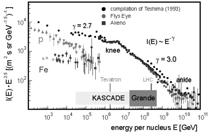
Fig. 1 - The energy spectrum of primary cosmic rays integrated on all particle species
