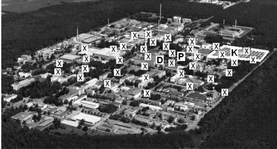
Fig. 2 - The KASCADE-Grande detector array with its components: the KASCADE array (K - the upper right rectangular area), the Digital Acquisition Station (D), the Grande stations (X), the Piccollo trigger array (P).
