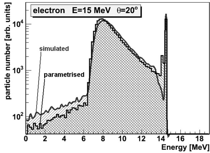
Fig. 5 - Example: comparison between simulated energy deposits and parametrised energy deposits for photons and electrons with a  $20^\circ$  angle of incidence
