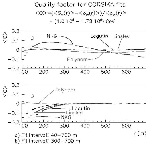
Fig. 7 - Example: Comparison of the reproduction of the average CORSIKA lateral charged particle distribution by various forms of the LDF (case : proton induced EAS of (1.0-1.78) ·10<sup>17</sup> eV)
