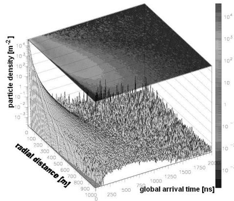
Fig. 3 - Structure of the EAS front for all EAS components
