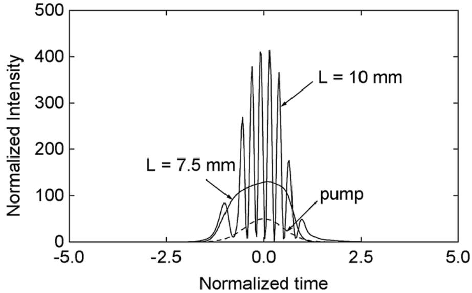
Fig. 10 – Intensity profile of the emerging signal for two different crystal lengths indicated with the arrows. The parameters correspond to point A in Fig. 1(b) and the reflectivity is  $R = 0.96$ . The intensity of the 1 ps pump pulse is  $I_p = 0.4 \text{ GW/cm}^2$ .
