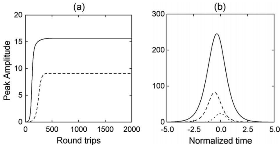
Fig. 3 – (a) Signal peak amplitude as a function of round trip number for two values of the mirror reflectivity. The input pump intensity is  $I_p = 0.8 \text{ GW/cm}^2$ . (b) Normalized intensity of the output signal (after 2000 round trips). The dotted line corresponds to the pump intensity profile. In both figures the solid lines correspond to  $R = 0.99$  and the dashed lines to  $R = 0.96$ . We have taken the parameters corresponding to the point A in Fig. 1(b).
