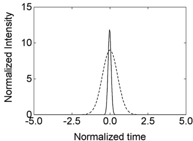
Fig. 5 – Intensity profile *versus* normalized time. Full line: Signal after 10000 round-trips, dashed line: 4 ps input pump. The parameters correspond to the point A in Fig. 1(b). Here  $I_p = 0.3$  GW/cm<sup>2</sup>, and  $R = 0.96$ .
