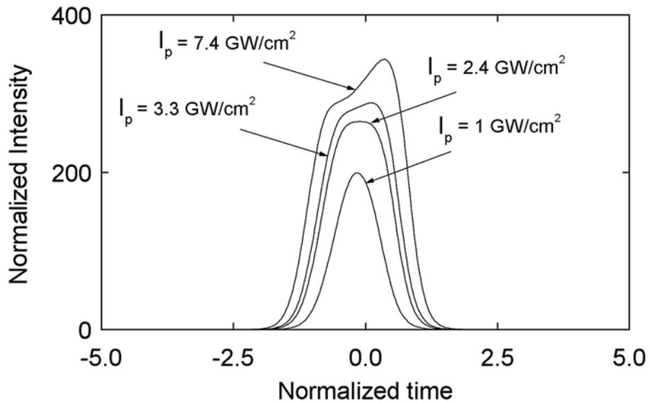
Fig. 11 – Intensity profile of the emerging signal for four different pump intensities indicated with the arrows. The parameters correspond to point A in Fig. 1(b), the reflectivity is  $R = 0.96$ , the pump duration is 300 fs and the crystal length is  $L = 2.5 \text{ mm}$ .
