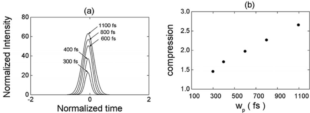
Fig. 4 – (a) Signal intensity profile for different pump durations, indicated with the arrows. Here  $I_p = 0.4$  GW/cm<sup>2</sup>, the reflectivity  $R = 0.96$ , and the other parameters correspond to the point A in Fig. 1(b). (b) Compression coefficient *versus* pump duration for the same parameters as above.
