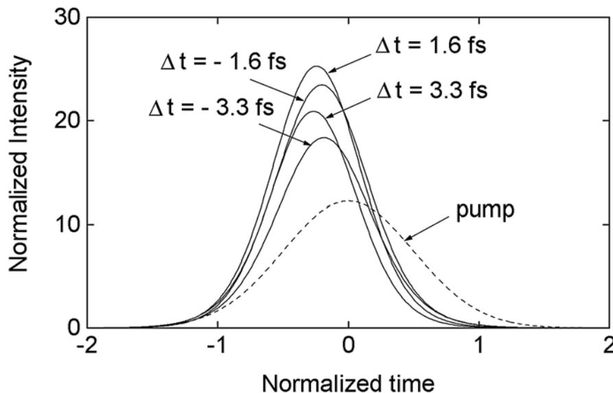
Fig. 12 – Signal intensity profile for various desynchronizations  $\Delta t$  between pump and signal waves. The parameters correspond to point A in Fig. 1(b), the reflectivity is  $R = 0.96$ , the pump duration is 300 fs, the pump intensity is  $I_p = 0.4 \text{ GW/cm}^2$  and  $L = 2.5 \text{ mm}$ .
