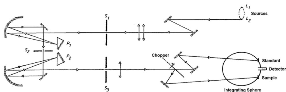
Fig. 2 – Experimental set up. Cary spectrophotometer and the Sphere.
