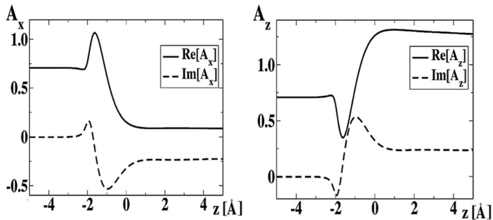
Fig. 3 – Variation with  $z$  of the spatial part of the vector potential near the interface for aluminium at oblique incidence of 15 degrees, for a laser of 2 eV, 30 J/m<sup>2</sup>: left side represents the tangential ( $x$ ) component and right side the normal ( $z$ ) one.
