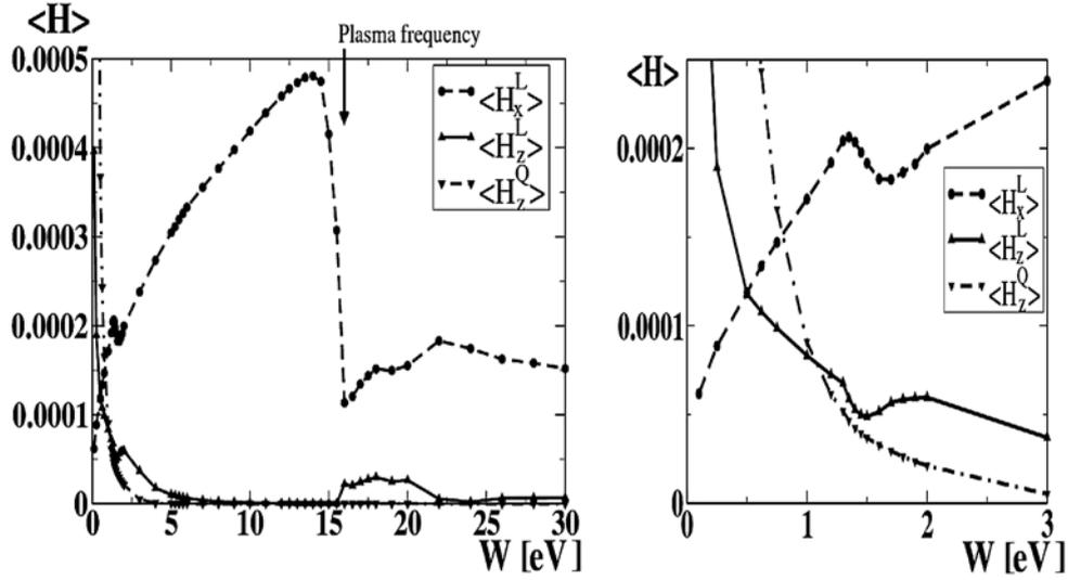
Fig. 4 – Expectation values for the linear terms  $\langle \hat{H}_z^L \rangle$ ,  $\langle \hat{H}_x^L \rangle$  and quadratic term  $\langle \hat{H}_z^Q \rangle$  of metallic aluminium for a  $p$  polarized laser, as function of laser energy for: left panel, whole energy range and right panel, low energy range.
