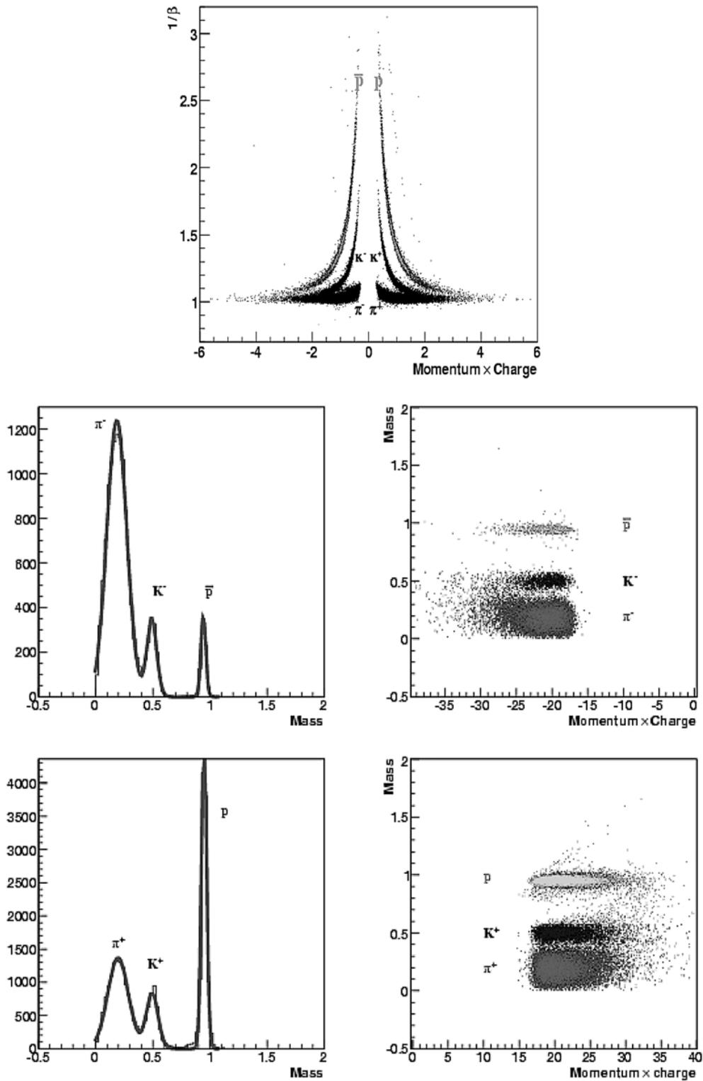
Fig. 1 – Left panel: particle identification in the MRS using TOFW, in which  $1/\beta = \sqrt{1 + m^2/p^2}$ , right panel: particle identification in the FS by RICH, the hadron mass ( $\text{GeV}/c^2$ ) vs. momentum  $\times$  charge ( $\text{GeV}/c$ ) were used. Right-upper and right-lower plots stand for the settings at 4 degree with A and B polarities correspondingly under full magnetic field.
