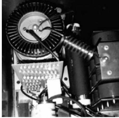
Fig. 15 – Photo illustrating Tor Vergata power inductor for LC-inversion in series with thyatron anode, L_o=524\text{nH} ; final computation has given, with d=23\text{mm} , l=40\text{mm} , loop spacing d_s=3.87\text{mm} , F=0.0116 : n_{Lo}\cong 7 turns. Spacing d_s is needed for maintaining electrically isolated the loops with a proper thickness of oil. Measured inductance is 537\text{nH} .
