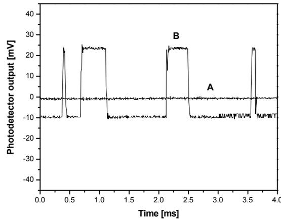
Fig.3 – Photodetector output voltage during modes hopping. Trace B show laser intensity switching between two intensities as the laser switch between the modes. The parameters used in measurements:  $I_{LD} = 56.8\text{mA}$ ,  $P_{out} = 2.2\text{mW}$ ,  $t = 30^{\circ}\text{C}$  for trace A and  $I_{LD} = 59\text{mA}$ ,  $P_{out} = 2.6\text{mW}$ ,  $t = 30^{\circ}\text{C}$  for trace B. The oscilloscope was a.c. coupled.
