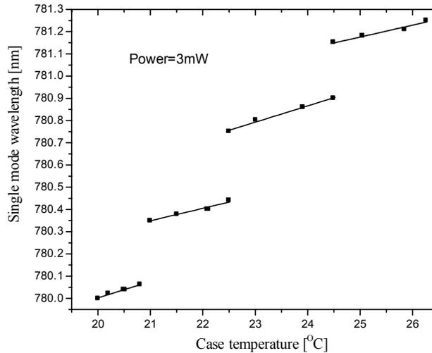
Fig.2 – Temperature dependence of single mode laser diode wavelength at constant emitted power. Continuous tuning range has a slope  $\sim 0.06 \text{ nmK}^{-1}$  while the discrete jumps of the wavelength are around 0.3 nm.
