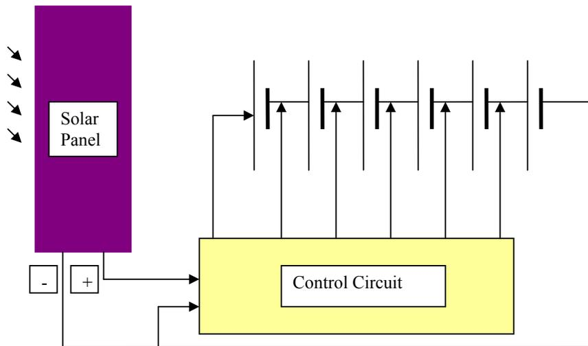
Fig. 3 – Block diagram of the controlled charging process.
