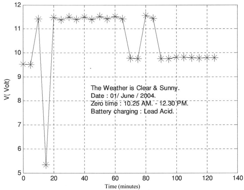
Fig. 8 – Controller voltage during lead-acid battery charging.
