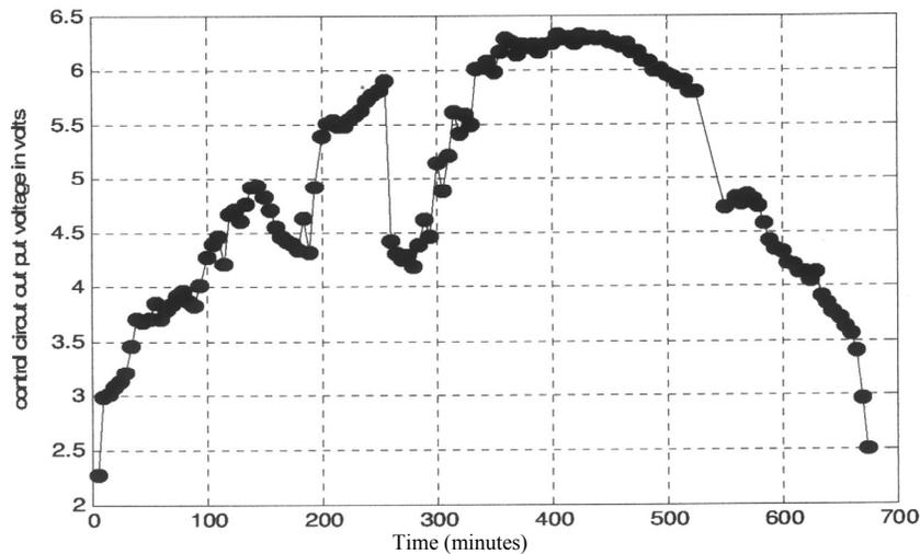
Fig. 6 – Controller voltage during nickel-cadmium battery charging.
