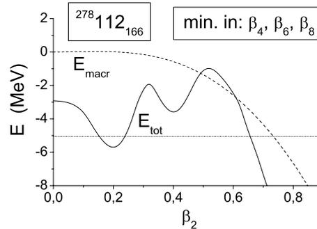
Fig. 1 – Static spontaneous-fission barrier calculated for the nucleus  $^{278}_{112}$  in the two cases: when only the macroscopic ( $E_{\text{macr}}$ ) and when the total ( $E_{\text{tot}}$ ) energy of it is considered [25].
