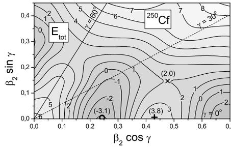
Fig. 3 – Contour map of the total potential energy calculated for the nucleus  $^{250}\text{Cf}$ . Numbers at the contour lines specify the value of the energy. Position of the saddle point is marked by the symbol “+”, when the axial symmetry of the nucleus is assumed, and by the symbol “x”, when non-axiality is taken into account. Position of the equilibrium point is denoted by the sign “o”. Numbers in parentheses give values of the energy at these points [28].
