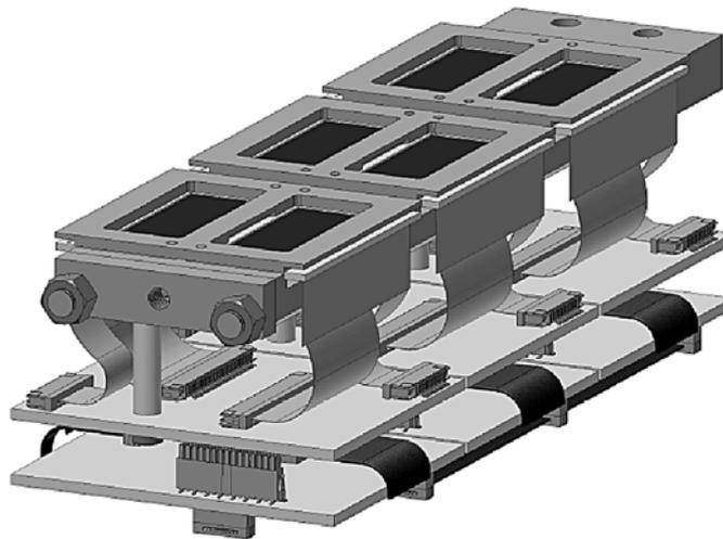
Fig. 6 – An 18 cm<sup>2</sup> SDD unit, containing 18 SDD individual chips.
