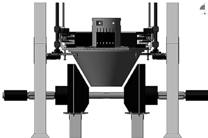
Fig. 9 – The schematic drawing of the SIDDHARTA setup in the Interaction Region of DAΦNE.
