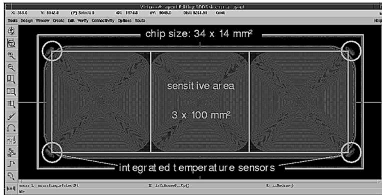
Fig. 5 – SDD layout on the readout side: 3 SDD cells, read independently, each of 1 cm<sup>2</sup> area, monolithically integrated on one chip.
