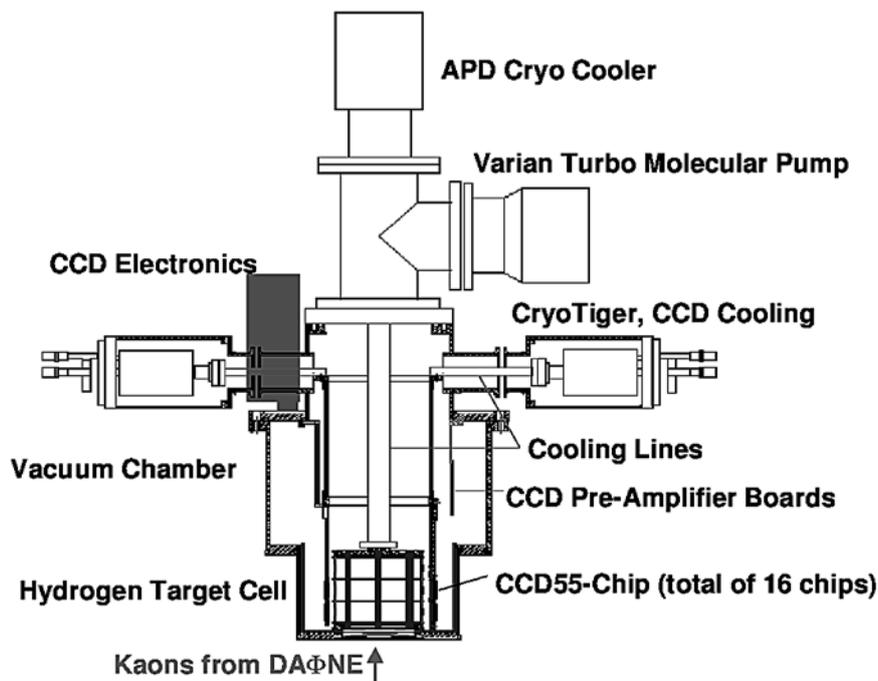
Fig. 2 – Schematic representation of the DEAR setup.
