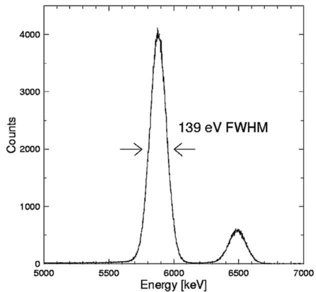
Fig. 7 – The X-ray spectrum from an Iron source as measured in the laboratory with an SDD chip prototype. The experimental resolution, FWHM (Full Width Half Maximum) at 5.9 keV is 139 eV.
