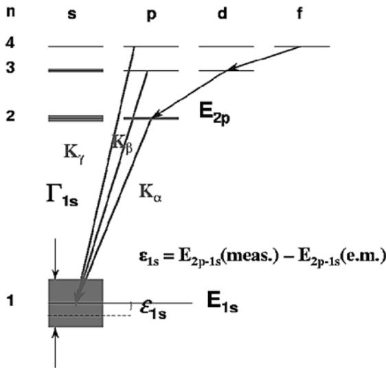
Fig. 1 – The cascade process in kaonic atoms with the shift and the broadening of the  $1s$  level, with respect to the purely electromagnetic calculated value, due to the presence of the strong interaction.
