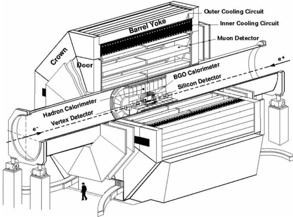
Fig. 1 – A general view of the L3 detector [3].
