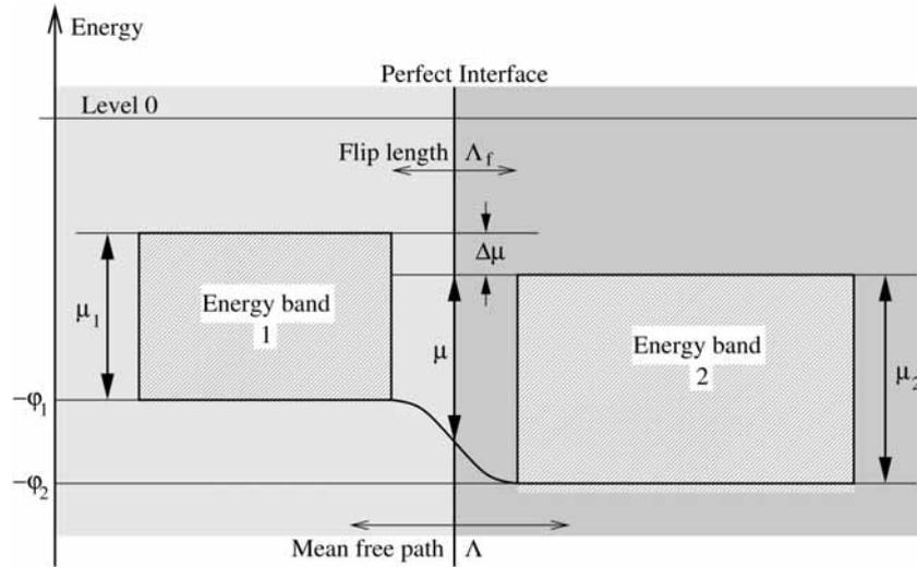
Fig. 1 – Two solids with a perfect contact.
