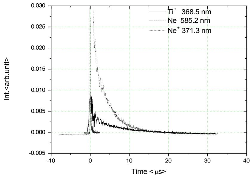
Fig. 2 - The emission profile of Ne, Ne<sup>+</sup> and Ti<sup>+</sup> spectral lines.
