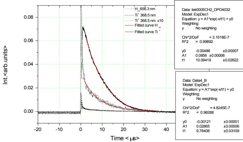
Fig. 3 - The emission lines of Ti<sup>+</sup> and H<sub>α</sub> and the corresponding fitting curves.
