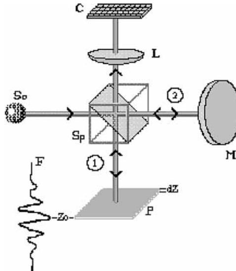
The CCD target ( $782 \times 582$  pixels) carries out simultaneously the measurement of all the points on the measured surface. There is no need to mechanical scanning along the  $x$  and  $y$  axes. This allows for small areas to be scanned with very high resolutions very quickly.
