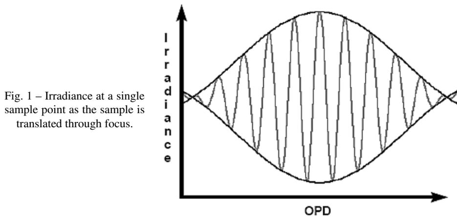
Fig. 1 – Irradiance at a single sample point as the sample is translated through focus.
