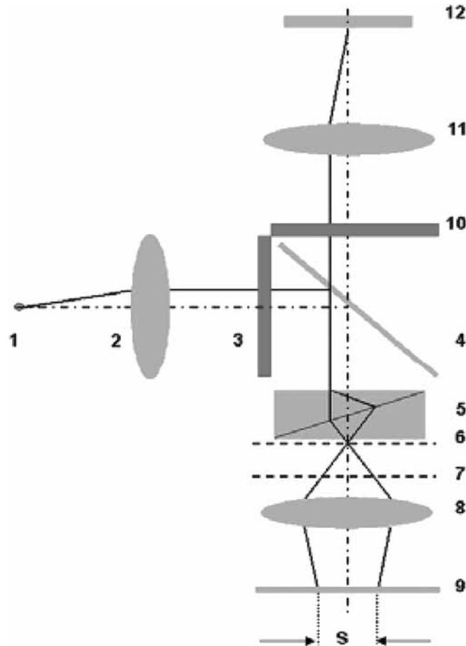
Fig. 7 – Schematic structure of the TIC shearing micro-interferometer.
