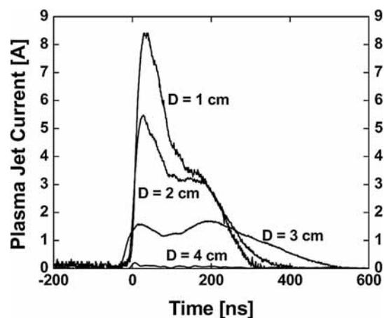
Fig. 3 – The plasma jet currents of the first generator configuration (Fig. 1a), for different distances ( $D$ ) from the plasma exit hole.
