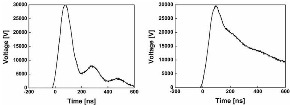
Fig. 2 – The high voltage pulses, obtained with the high voltage repetitive pulser: the primary capacitor = 5 nF (left), and 20 nF (right).
