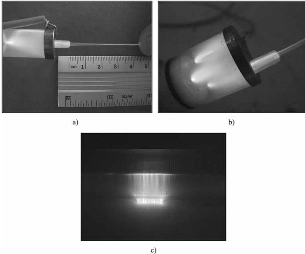
Fig. 1 – The geometrical configurations which have been tested for plasma jet generator: a) point-plate; b) multiple points-plate; c) wire-plate.
