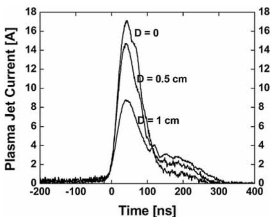
Fig. 4 – The plasma “curtain” currents of the wire-plate configuration (Fig. 1c), for different distances ( $D$ ) from the exit slit.
