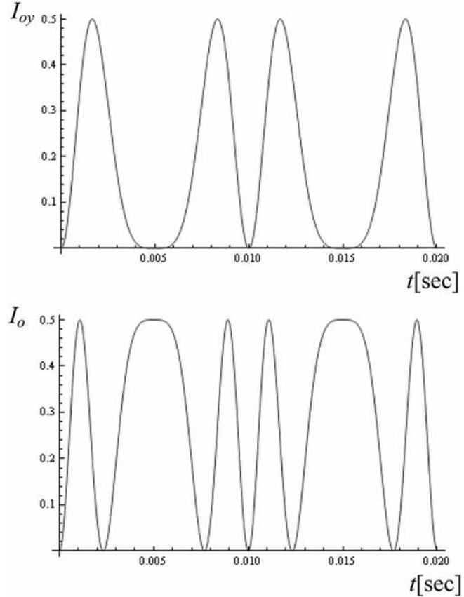
By increasing the amplitude of the input signal beyond a certain limit, a pair of symmetric “humps” appears in the time-varying form of the output (Fig. 4). Again, the exact value of this limit can be obtained by performing the temporal derivative of the output signal and by imposing on it to have a point of annullment on the first quarter-period (open interval):
