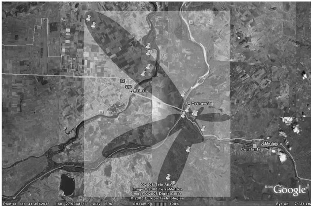
Fig. 4 – Assessing the 48-hour vulnerability induced by an accidental environmental release-in-process (of yet unknown duration) of radioactivity, at Cernavoda NPP. Pinpoints are GIS-linked and referred upon community sites. With RAT, such static images has *Google Earth* (TM) dynamic counterparts (KML files).
