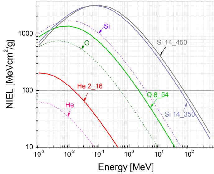
Fig. 2 – Non-ionizing energy loss *versus* energy in silicon for ordinary ions:  ${}^4_2\text{He}$ ,  ${}^{16}_8\text{O}$ ,  ${}^{28}_{14}\text{Si}$  and for the strangelets:  ${}^{16}_2\text{He}$ ,  ${}^{54}_8\text{O}$ ,  ${}^{350}_{14}\text{Si}$ , and  ${}^{450}_{14}\text{Si}$ .
