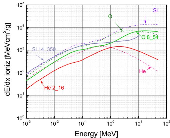
Fig. 1 – Ionization energy loss *versus* energy in silicon for ordinary ions:
