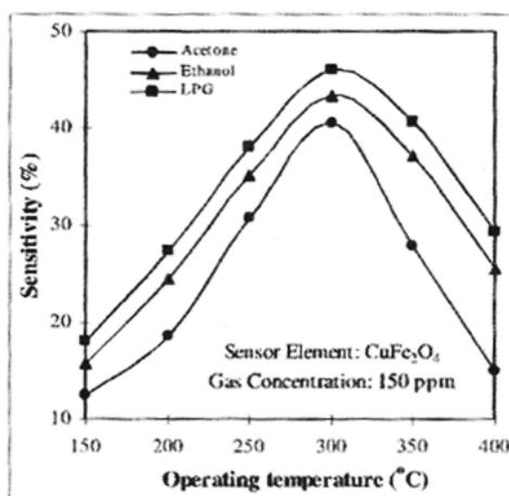
Fig. 3 – Variation of gas sensitivity as a function of operating temperature for  $\text{CuFe}_2\text{O}_4$  sensor element.
