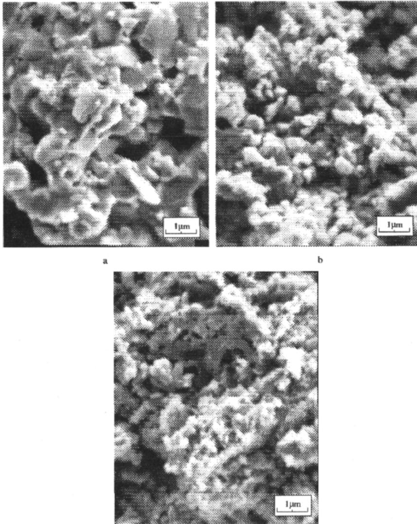
Fig. 2 – SEM micrographs of the  $\text{CuFe}_2\text{O}_4$ (a),  $\text{CdFe}_2\text{O}_4$ (b) and  $\text{ZnFe}_2\text{O}_4$ (c) ferrites. Enlargement  $\times 8000$ .
