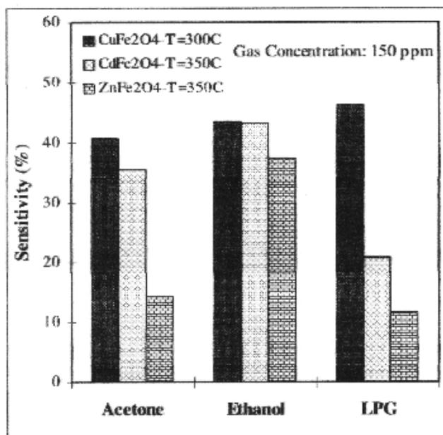
Fig. 6 – Bar diagram for maximum sensitivities to test gases of CuFe<sub>2</sub>O<sub>4</sub>, CdFe<sub>2</sub>O<sub>4</sub> and ZnFe<sub>2</sub>O<sub>4</sub> ferrites.
