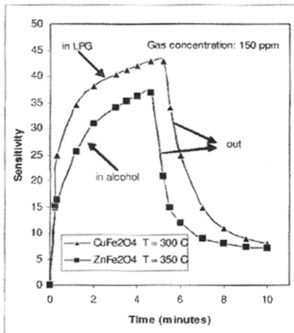
Fig. 8 – Response characteristics to LPG for  $\text{CuFe}_2\text{O}_4$  and to ethanol for  $\text{ZnFe}_2\text{O}_4$ .
