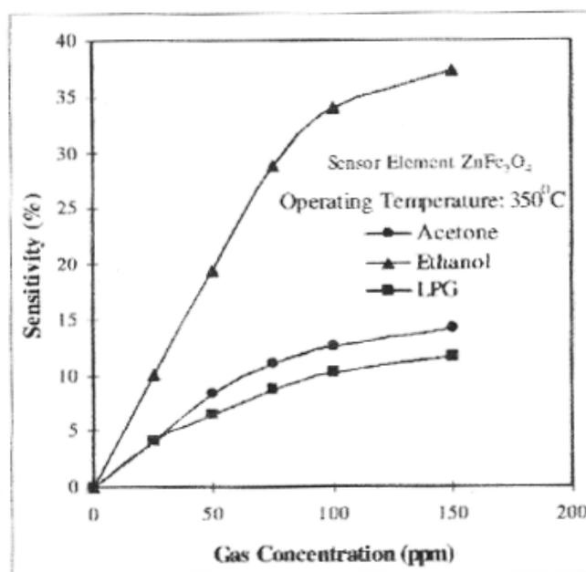
Fig. 7 – Gas sensitivity *versus* gas concentration of  $\text{ZnFe}_2\text{O}_4$  sensor element.
