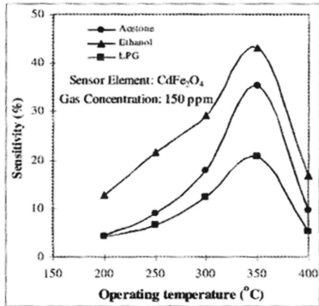
Fig. 4 – Variation of gas sensitivity as a function of operating temperature for  $\text{CdFe}_2\text{O}_4$  sensor element.
