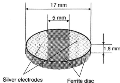
Fig. 1 – Design of ferrite sensor with silver electrodes.
