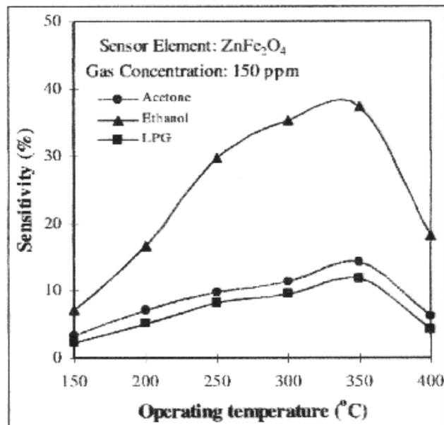
Fig. 5– Variation of gas sensitivity as a function of operating temperature for  $\text{ZnFe}_2\text{O}_4$  sensor element.
