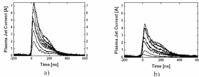
Fig. 3 – The current of the plasma jet at a distance of 1 cm (a) and 2 cm (b) from the exit outlet, for various concentrations of oxygen in helium (He – 4 l/min). From the most intense to the weakest current, the oxygen concentrations are: 0.2 %; 0.4 %; 0.6 %; 0.8 %; 1 %; 1.5 %; 2 % respectively.
