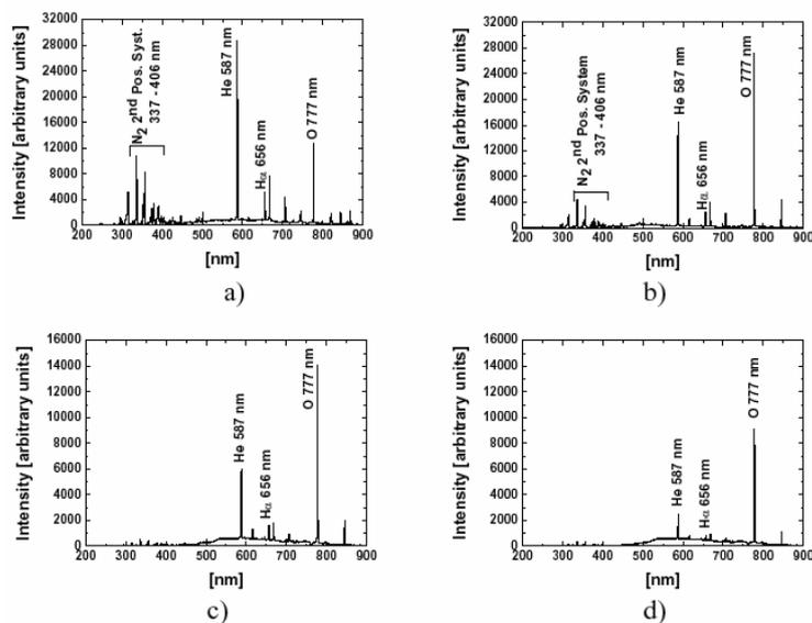
Fig. 5 – Emission spectra of the helium plasma jets (5 l/min), for various values of the concentration of the oxygen introduced in the discharge area: a) 0 %; b) 0.5 %; c) 1 %; d) 1.5 %.
