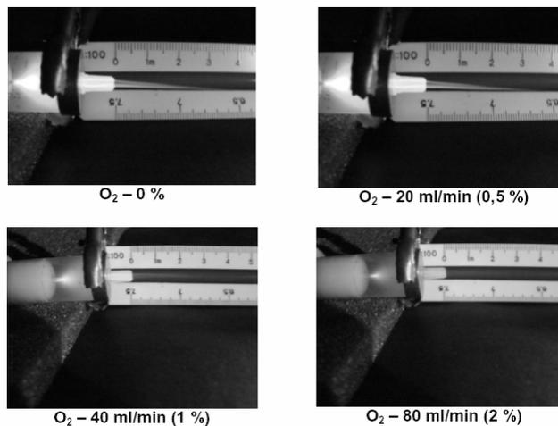
Fig. 4 – Oxygen chemical activation (He – 4 l/min). Discharge between electrodes, and plasma jet for various concentrations of oxygen in helium. Chemical activation of the high voltage pulsed, cold atmospheric plasma jets
