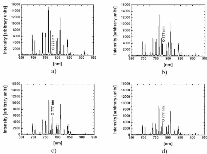
Fig. 6 – Emission spectra of the argon plasma jets (2 l/min), for various values of the concentration of the oxygen introduced in the discharge area: a) 0 %; b) 0.5 %; c) 1 %; d) 1.5 %.
