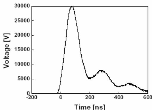
Fig. 1 – High voltage pulse, obtained with the high voltage repetitive pulser.
