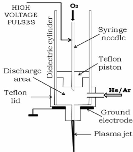
Fig. 2 – Drawing of the device for generating high voltage pulsed, cold atmospheric plasma jets.
