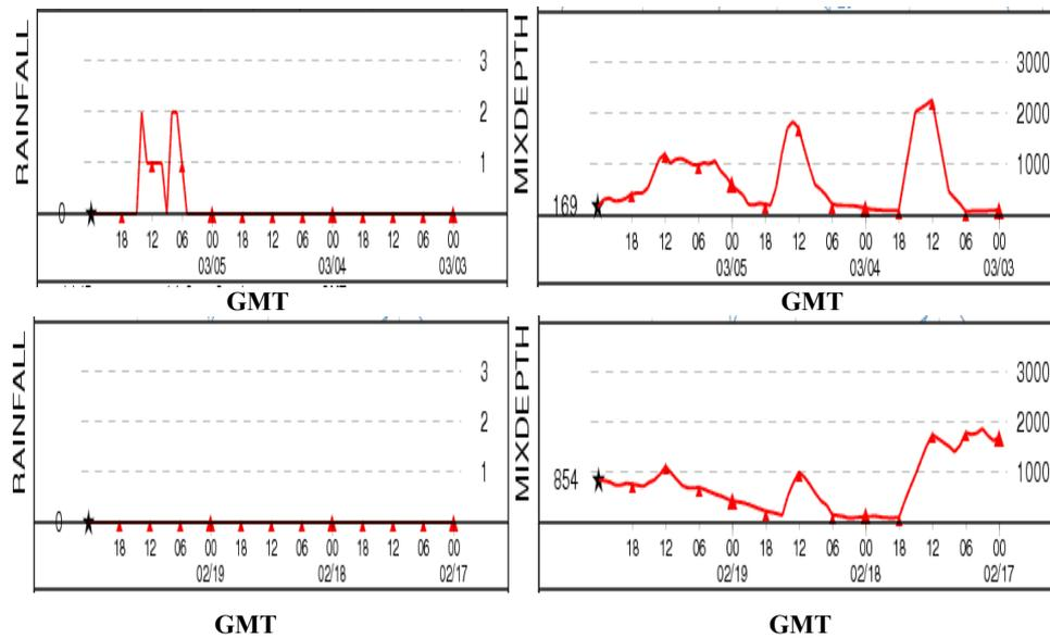
Fig. 3 – Meteorgrams obtained using HYSPLIT 4 [9]: precipitation left column and mixed layer height on right column; upper panel 05<sup>th</sup> of March 2009 and lower for 19<sup>th</sup> of February 2009.
