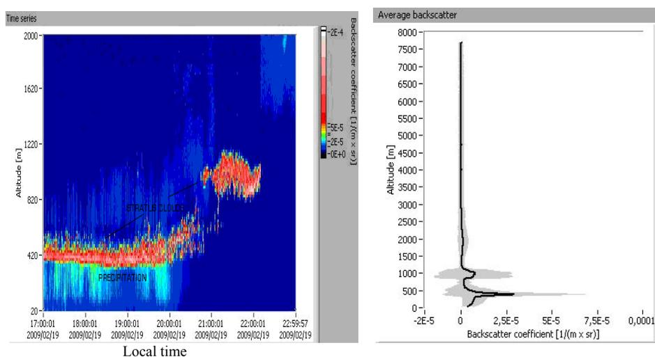
Fig. 2 – As in Fig. 1 but for 19<sup>th</sup> of February 2009 in evening hours. In backscatter profile can be observed the two levels of the PBL marked by the cloud bases.
