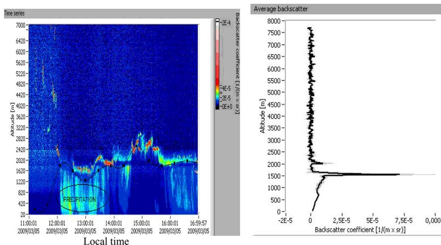
Fig. 1 – Image of the PBL (left) and associated backscatter profile (right) for 05<sup>th</sup> of March 2009. The solid curve marks out the mixed layer height; the period with precipitation is also marked. The backscatter profile shows the mixed layer at the same height as in image (appropriate on 1500m).
