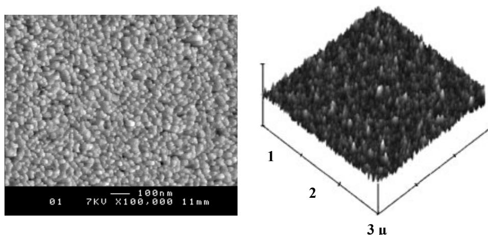
Fig. 1 – FSEM (left) and AFM (right) pictures of rough Au support.
