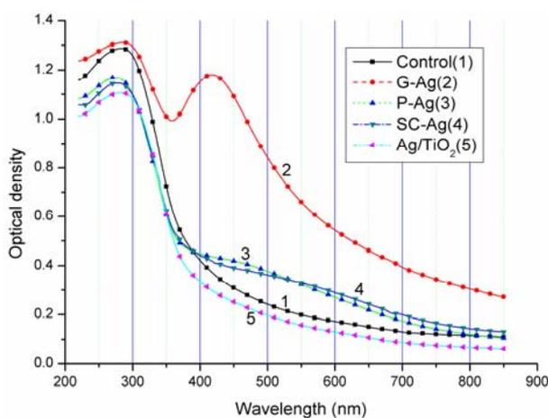
Fig. 1 – Absorption spectra of leather samples obtained by diffuse reflection measurements.
