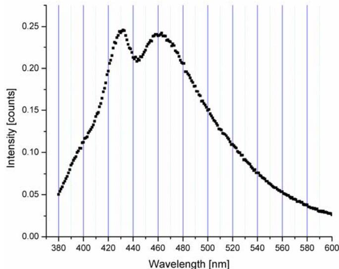
Fig. 3 – Fluorescence emission spectrum of genuine leather sample.
