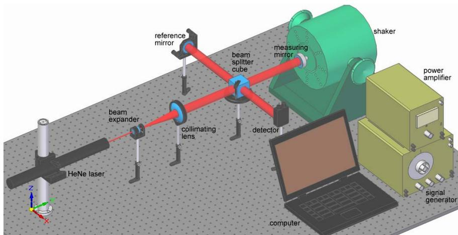
Fig. 2 – 3D representation of the experimental setup.
