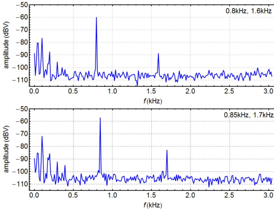
Fig. 4 – Recorded spectra for the vibrations having resonance frequencies of 0.8 and 0.85 kHz. The 2<sup>nd</sup> harmonic peaks do not appear anymore as we reduced them by decreasing the amplitude of vibration.
