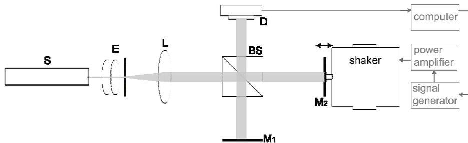
Fig. 1 – Experimental setup: S – HeNe laser source, E – beam expander, L – collimating lens, BS – beam splitter,  $M_1$  – reference mirror,  $M_2$  – measuring mirror, D – photo detector, shaker, signal generator, power amplifier and computer.
