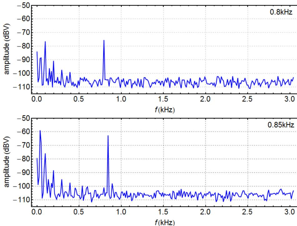
Fig. 5 – Recorded spectra for the vibrations having resonance frequencies of 0.8 and 0.85 kHz. Both the 1<sup>st</sup> and 2<sup>nd</sup> harmonics were reduced to zero.
