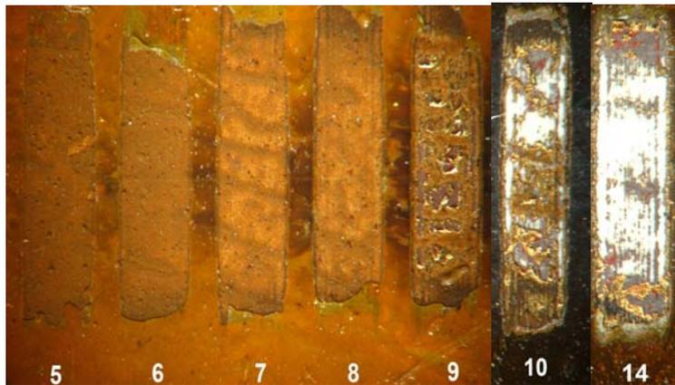
Fig. 2 – Sequence of laser removal of painting layers. Irradiation conditions: wavelength 355 nm; incident fluence  $90 \text{ mJ/cm}^2$ ; subsequent irradiation pulses number (from left to right) 7, 10, 15, 20, 30; 5 sec., 60 sec.; the corresponding measured ablation depth was 15, 18, 21, 23, 25, not measured, 45  $\mu\text{m}$ .
