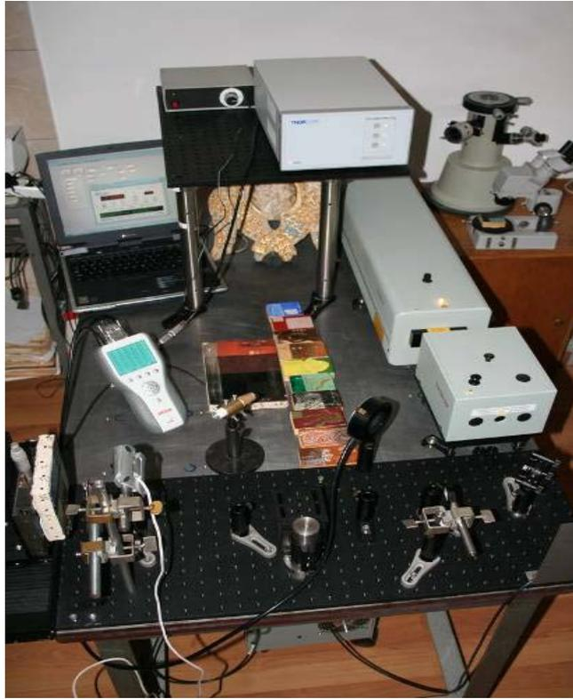
Fig. 1 – General view of the experimental set-up developed for laser cleaning experiments.
