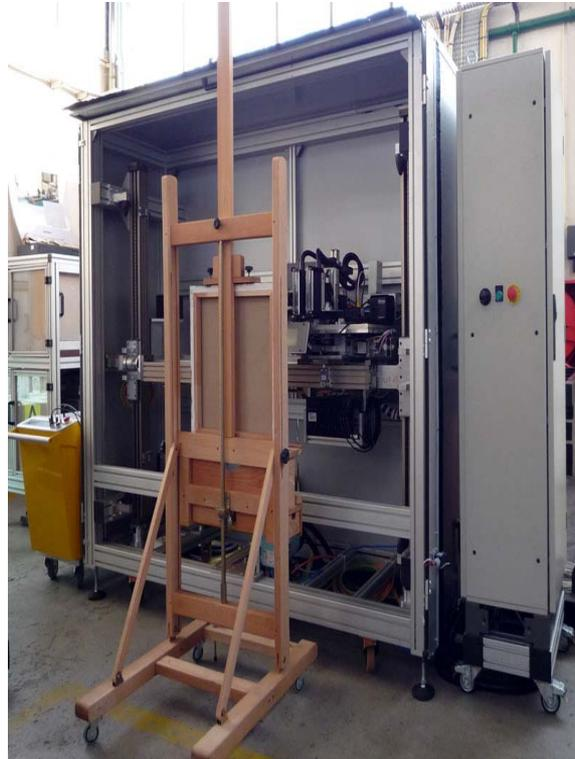
Fig. 6 – Laser cleaning prototype general image.
