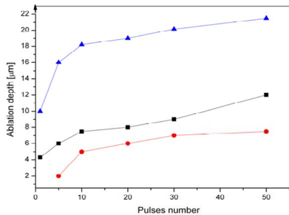
Fig. 5 – Ablation depth evolution as a function of subsequent irradiation pulse number for 3 incident fluences: 30 mJ/cm<sup>2</sup> – ● line, 90 mJ/cm<sup>2</sup> – ■ line, 200mJ/cm<sup>2</sup> – ▲ line (Mock-up: Support: WOOD; Substrate: ground powder of chalk with finings; layers: natural sienna iron rust, white and pink all in tempera egg emulsion 1/4, mastic varnish 12%, Patina and dummy dirt\*: Opaque layer: Mixture of powder of chalk +plaster + black smoke + finings-4%).
