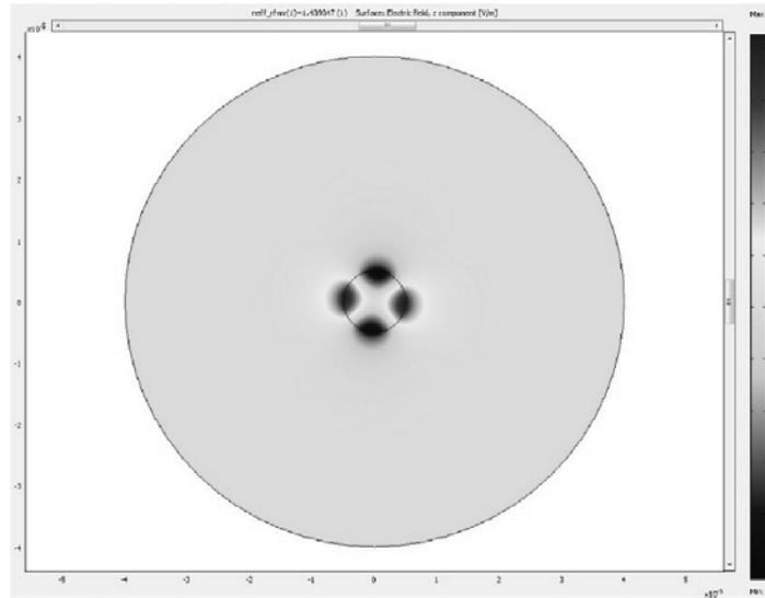
Fig. 4 – The numerical simulated time averaged laser electric field distribution into the transverse section of a singlemode optical fiber with a core of  $10\ \mu\text{m}$  diameter and a cladding of an  $80\ \mu\text{m}$  overall diameter.
