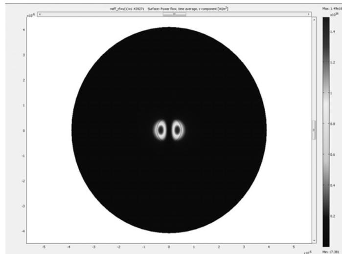
Fig. 5 – The numerical simulated time averaged laser power flow across the transverse section of a singlemode optical fiber with a core of  $8.82\ \mu\text{m}$  and  $11.33\ \mu\text{m}$  axes and a cladding of  $70.59\ \mu\text{m}$  and  $90.67\ \mu\text{m}$  axes.
