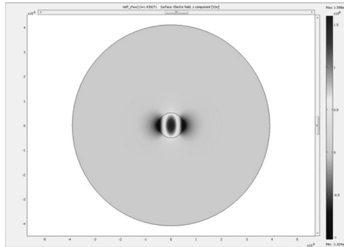
Fig. 6 – The numerical simulated time averaged laser electric field distribution into the transverse section of a singlemode optical fiber with a core of 8.82  $\mu\text{m}$  and 11.33  $\mu\text{m}$  axes and a cladding of 70.59  $\mu\text{m}$  and 90.67  $\mu\text{m}$  axes.
