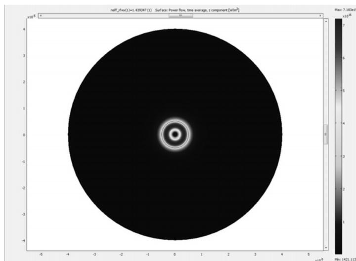
Fig. 3 – The numerical simulated time averaged laser power flow across the transverse section of a singlemode optical fiber with a core of  $10\ \mu\text{m}$  diameter and a cladding of an  $80\ \mu\text{m}$  overall diameter.
