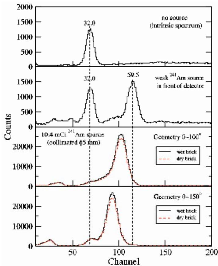
Fig. 2 – Region of the spectra obtained with the lanthanum bromide detector under different conditions.
