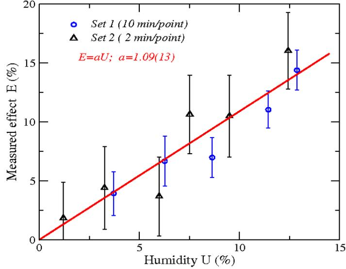
Fig. 5 – Comparison between two sets of measurements on the same type of bricks: the one from Fig. 4 (measuring time 10 min/point) and another one with 2 min/point. The line is the fit to all 11 data points.
