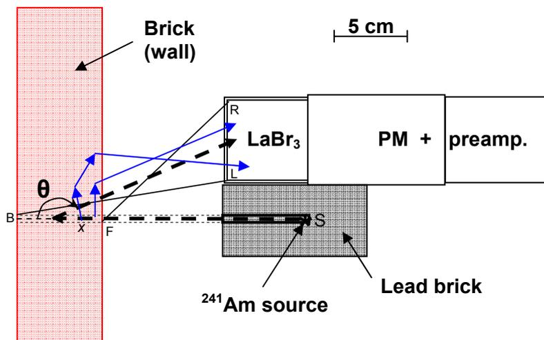
Fig. 1 – Sketch of the experimental setup used in the present measurements. Both single scattering and multiple-scattering processes are illustrated.
