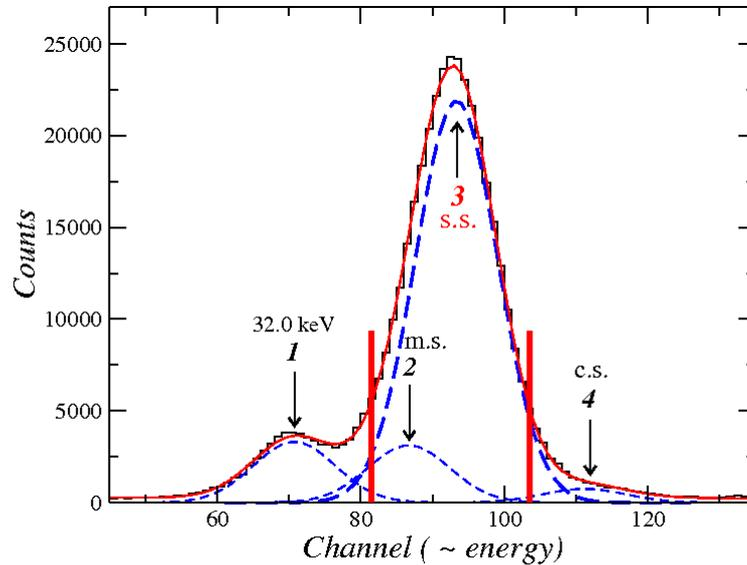
Fig. 3 – Example of gaussian peak decomposition of a scattered spectrum in the geometry of Fig. 1. The peaks have the following energies: no. 1: 32 keV; no. 2: 45.0 keV; no. 3: 48.7 keV (the single Compton scattering peak); no. 4: 58 keV. The two markers show the limits of the peak integration discussed in the text.
