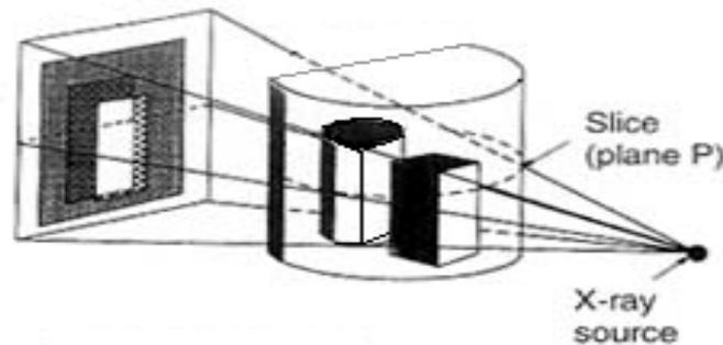
Fig. 1 – A conventional X-ray and a CT image acquisition.
