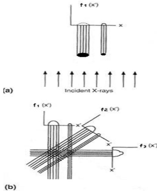
Fig. 2— a) Attenuation measurement at a given angle for a single view  $f(x')$ , where  $x'$  shows the linear position of it; b) back projections.
