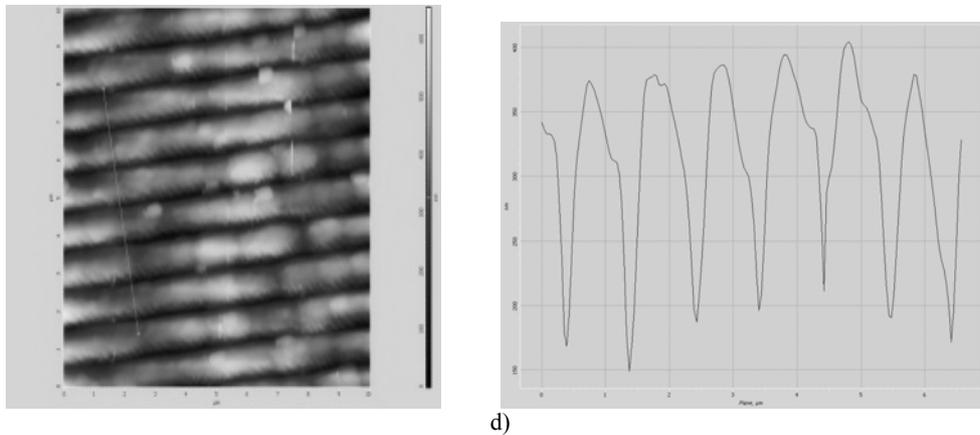
Fig. 3 – Surface relief evolution as a function of irradiation pulses number; material: photoresist AZ 5214E; irradiation wavelength 193 nm. Induced structure: grating with 1  $\mu\text{m}$  pitch; irradiation conditions: fluence 5  $\text{mJ}/\text{cm}^2$ ; pulse number/modulation depth: a) 2 pulses / 30–35 nm; b) 4 pulses / 40–70 nm; c) 8 pulses / 60–80 nm; d) 20 pulses/180–200 nm.
