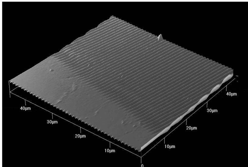
Fig. 1 – AFM image of the border of the single step SRG induced on the surface of the photoresist film under the action of 193 nm laser interference field.
