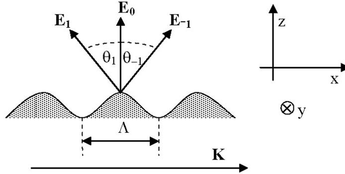
Fig. 6 –Experimental geometry and diffraction problem. The phase grating and the transmitted orders.  $\mathbf{K}$  is the grating vector indicating the direction of periodicity and having the scalar value of  $2\pi/\Lambda$ .  $\theta_{\pm 1} = \pm 11.13^\circ$ . The  $-1^{\text{st}}$  order is suppressed so that only the  $0^{\text{th}}$  and the  $+1^{\text{st}}$  orders contribute to the formation of the SRG.
