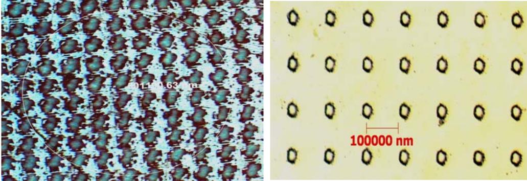
Fig. 5 – Surface relief structures induced on the photoresist film surface under the action of 355 nm laser light field.
