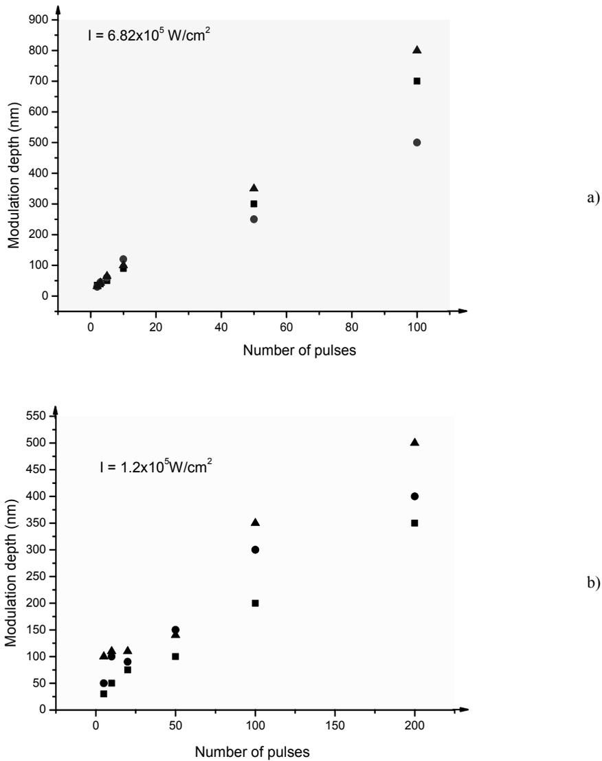
Fig. 4 – Single step surface relief gratings (1  $\mu\text{m}$  pitch) induced on photoresist film modulation depth dependence on subsequent irradiation pulses number for two fixed incident fluences; incident wavelength = 193 nm, film thickness: a) 2  $\mu\text{m}$  (▲), 1.5  $\mu\text{m}$  (■) and 1.2  $\mu\text{m}$  (●); b) 2  $\mu\text{m}$  (▲), 1.5  $\mu\text{m}$  (●), 1.2  $\mu\text{m}$  (■).
