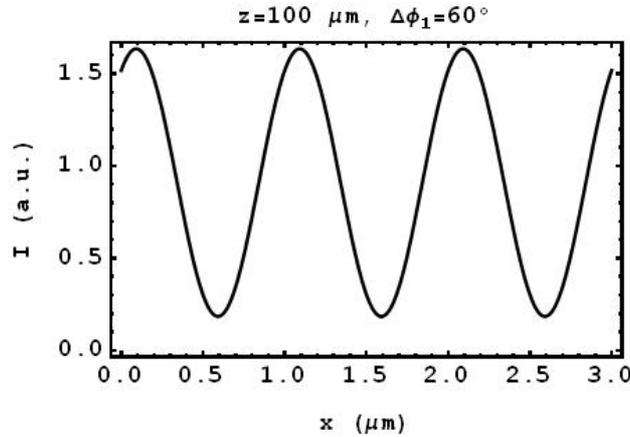
Fig. 7 – Interference sinusoidal pattern calculated for the  $1 \mu\text{m}$  pitch phase grating. The pattern does not depend on the distance  $z$  from the grating (as long as the distance is small enough) except for a phase shift of the sinusoid, which cannot be measured. The value of the  $\Delta\phi_1$  phase shift between the  $0^{\text{th}}$  and the  $1^{\text{st}}$  orders is also inconsequential.
