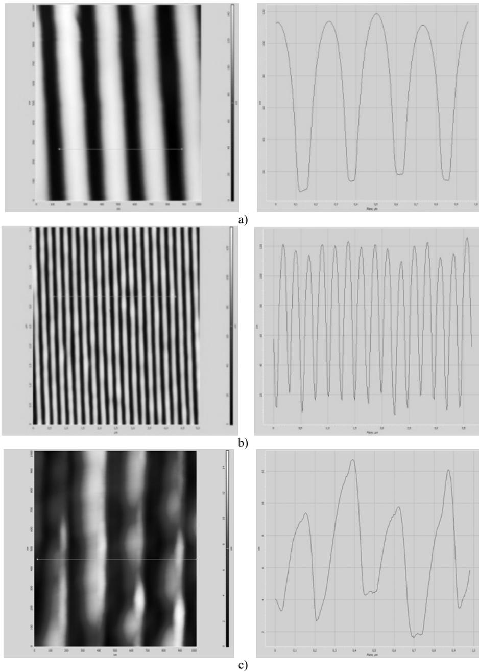
Fig. 2 – AFM image and profile of the 250 nm pitch surface relief grating obtained on the photoresist film (SU8.2). Irradiation conditions: irradiation wavelength – 193 nm, incident fluence –  $5 \text{ mJ/cm}^2$ , irradiation time / modulation depth: a) 4s / 105 nm; b) 4s / 90 nm; c) 1s / 7–9 nm.
