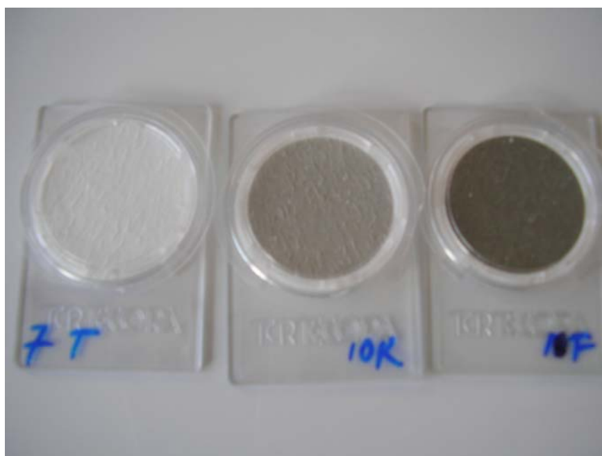
Fig. 1 – Quartz filters charged with PM10: 7T = blank filter, 10K = filter from blank area, 10F = filter from polluted area.
