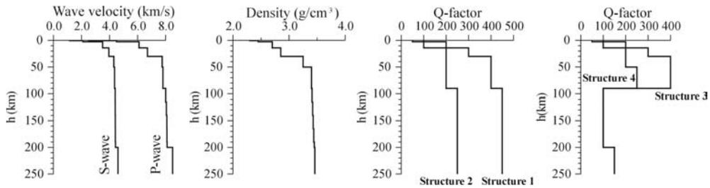
Fig. 6 – The structural models for the source – MAN station ray path.
