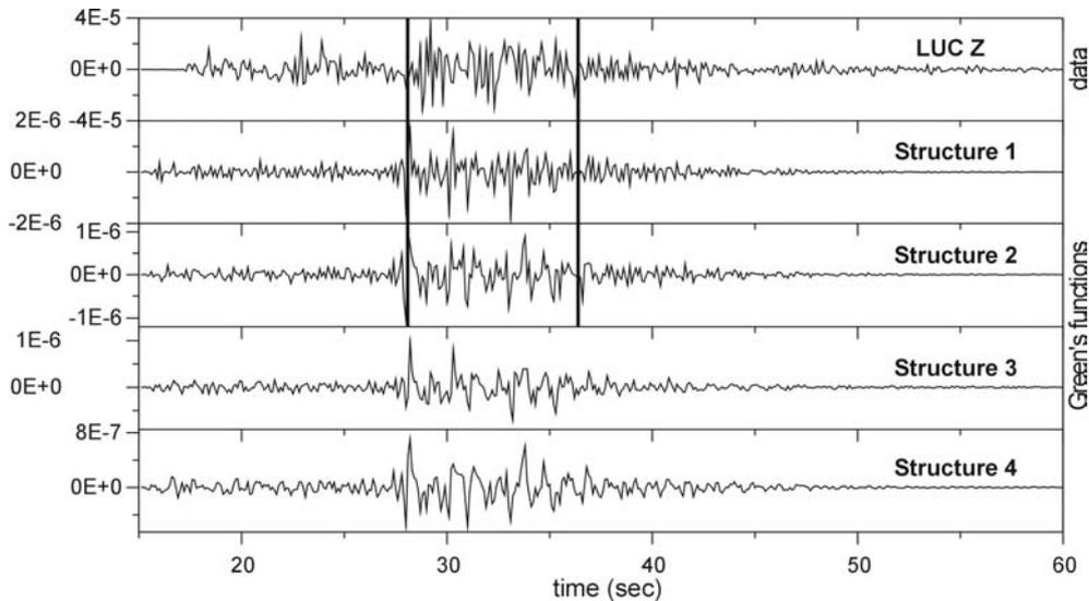
Fig. 10 – The selection of the time window. The observed data (m/s) are plotted together with the elementary seismograms (m/s), computed for several models for  $Q$ -factor. Elementary seismograms correspond to an instantaneous point source located in the hypocenter of the study earthquake, having the scalar moment  $M_0 = 10^{15}$  Nm, and based on a moment tensor with  $M_{11}$  the only nonzero component. Vertical bars indicate the time window used in the inversion.
