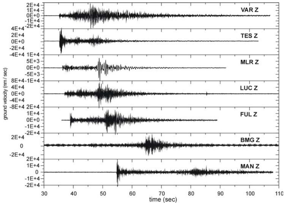
Fig. 2 – The observed waveforms - rough data; epicentral distances: VAR station – 70 km, TES station – 86 km, MLR station – 86 km, LUC station – 89 km, FUL station – 106 km, BMG station – 175 km, MAN station – 245 km.
