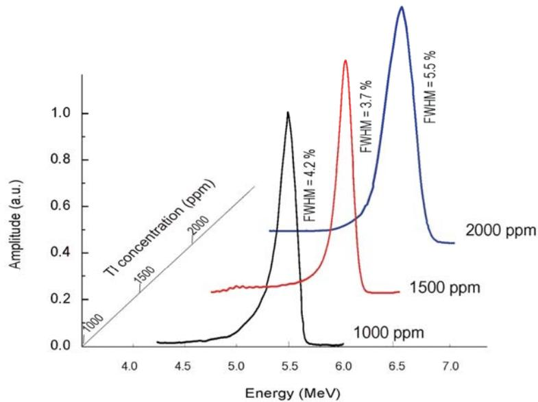
Fig. 1 – Energy spectrum of the 5.486 MeV line of  $^{241}\text{Am}$  SEA 4-2 alpha ray source obtained by using CsI(Tl) crystals with different content of Tl. All spectra were obtained in the same experimental conditions, but for a better comparison all were normalized to maximum amplitude. It is worth mentioning in all cases the maximum amplitude corresponded to the same channel.
