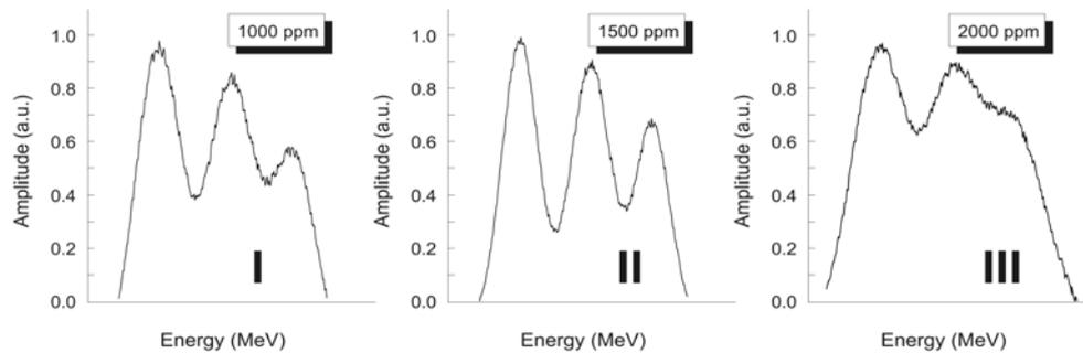
Fig. 2 – Energy spectra of the triple alpha source AMR 33 - R9207 ( $^{239}\text{Pu}$ ,  $^{241}\text{Am}$ ;  $^{244}\text{Cm}$ ) recorded by means CsI(Tl) scintillators with different content of Tl. The 1500 ppm Tl detector shows the best energy resolution (spectrum II).
