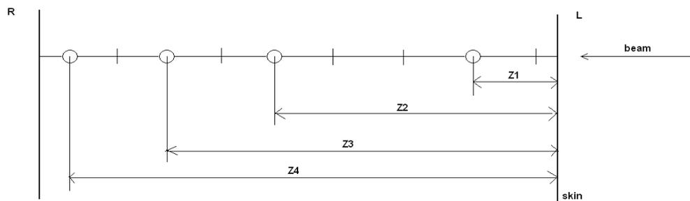
Fig. 1 – TLD's positions inside the Rando phantom on the central photons beam.  $z_i$  represent the distances between the patient skin and the TLD positions.
