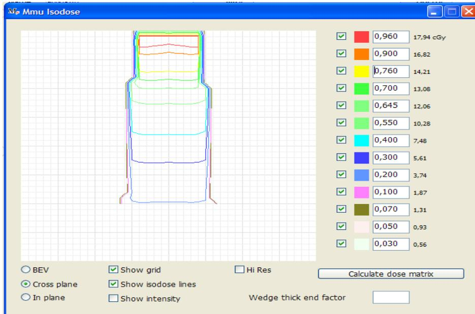
Fig. 2 – The isodose graphs and their values for Rando phantom exposure at 6 MeV photon beam and for 10 cm × 10 cm field.
