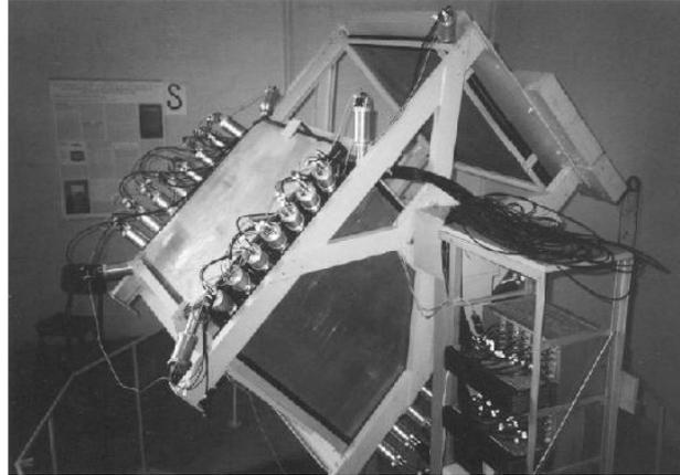
Fig. 3 – Rotatable WILLI detector [7].
