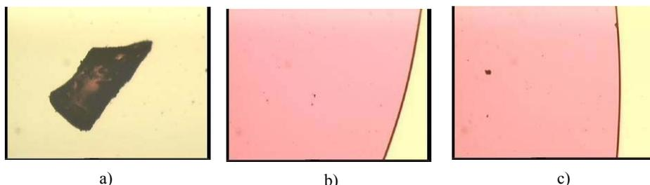
Fig. 7 – Optical images (between parallel polarizers) of a cell filled with the studied derivative at temperatures as follows: a) 24.8°C, during the heating; b) 90°C, during the heating; c) 37°C, during the cooling.
