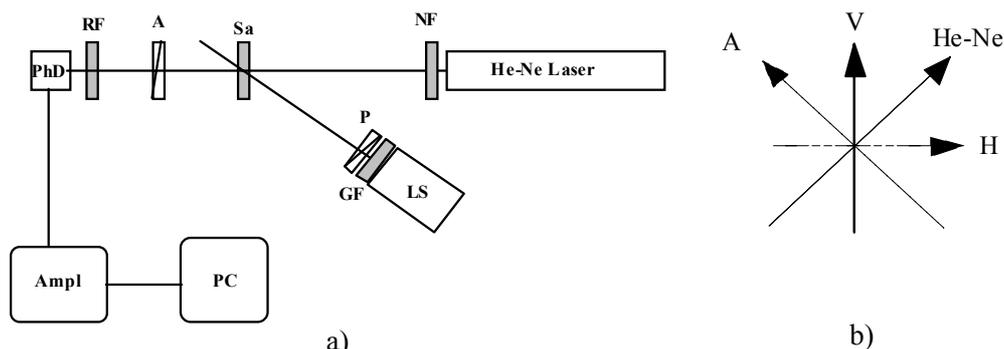
Fig. 2 – a) Sketch of the experimental setup: *NF* – neutral filter, *Sa* – sample, *A* – analyzer, *RF* – red filter, *PhD* – photodiode, *Ampl* – amplifier, *PC* – computer, *LS* – incandescent light source, *GF* – green filter, *P* – polarizer. b) Detail on the direction of the light polarization.
