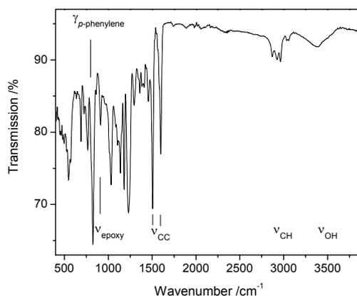
Fig. 5 – FTIR spectrum of the studied derivative and the assignment of main peaks.
