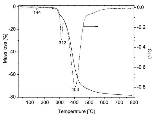
Fig. 3 – TG curve (continuous line) and its derivative DTG (dotted line) of the material.
