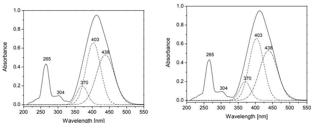
Fig. 6 – UV-Vis spectrum of the aminoazobenzene-epoxy resin derivative: a) in chloroform solution; b) comparison of the peak at ca 400 nm in the case of the sample solved in chloroform (1), deposited onto a glass plate (2) and deposited onto glass plate but after irradiation (3).
