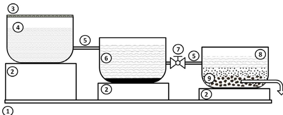
Fig. 4 – Small-scale model of the drinking water plant (a sketch performed by students in the project diary). The numbers in figure represent: 1) board, 2) supports, 3) sieve, 4) entry tank, 5) water pipes, 6) decantation tank, 7) control valve (tap), 8) final tank, and 9) sand and gravel filter.
