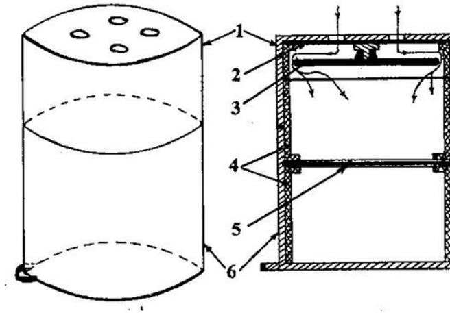
Fig. 1 – The radon monitoring device: general view and details: 1 – end cap with holes for radon entry; 2, 3, 4 – various holding elements for filter and SSNTD foil; 5 – SSNTD; 6 – end cap with ring.
