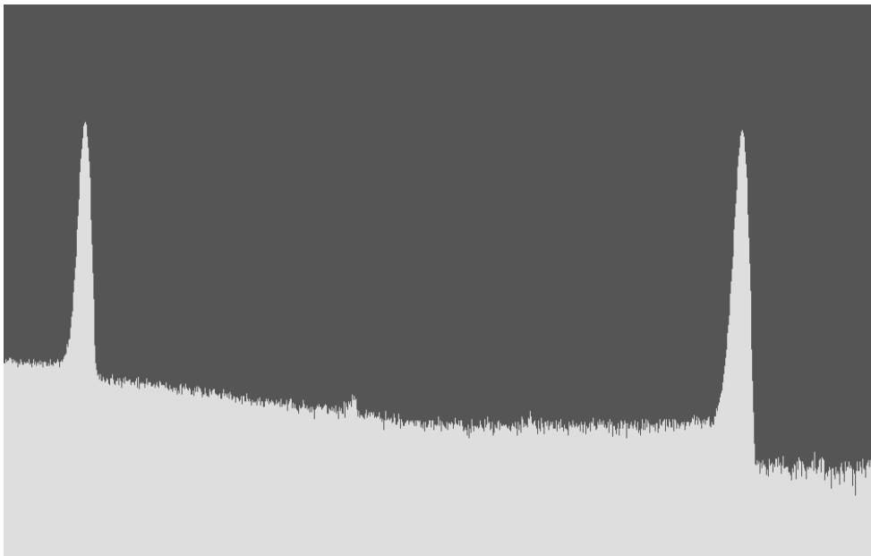
Fig. 1 – The high energy part of the ^{60}\text{Co} spectrum measured with the n-type detector in the absence of ^{133}\text{Ba} source. The dead time is about 0.3%.
