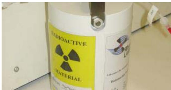
Fig. 1 –  $^{68}\text{Ge}/^{68}\text{Ga}$  generator.
