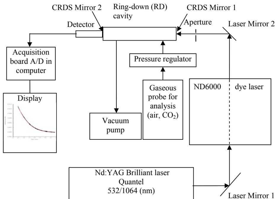
Fig. 1 – Experimental setup for CRDS of gaseous media.
