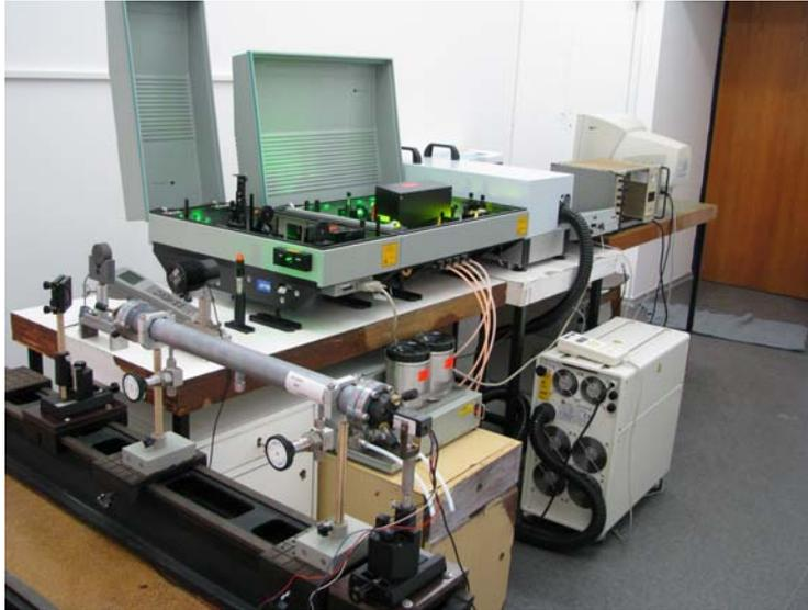
Fig. 2 – Experimental CRDS set-up for gaseous media.
