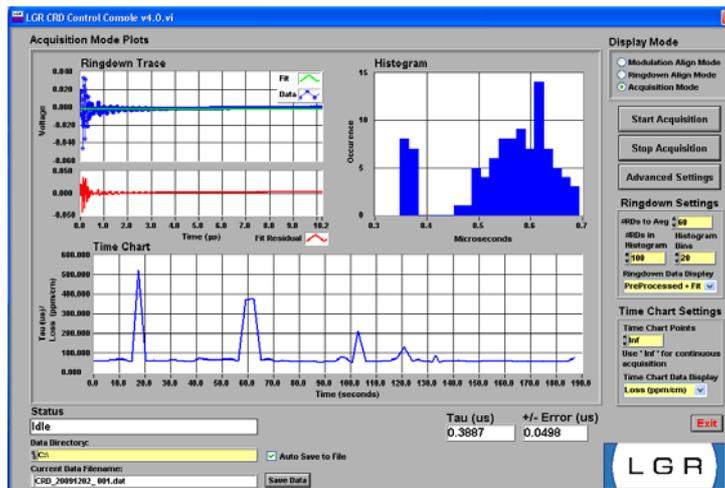
Fig. 10 – Loss registration at 1 064 nm in resonant cavity without  $\text{CO}_2$  in chosen working point, average ring-down time:  $0.52 \mu\text{s}$  and baseline:  $79.71 \text{ ppm/cm}$ .
