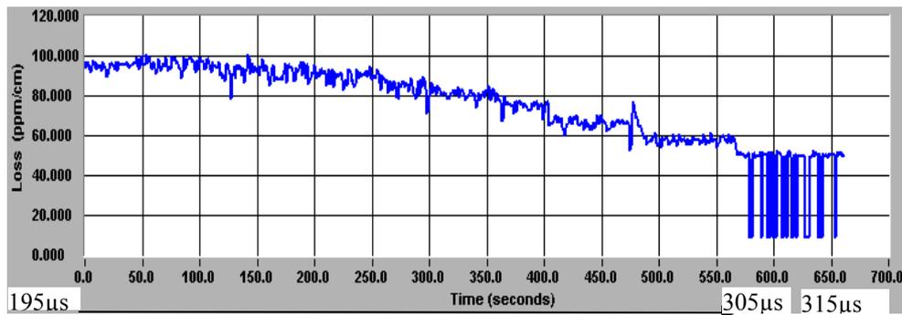
Fig. 5 – Total loss of resonant cavity with atmospheric air (baseline) at 1 bar in resonant cavity for a 660 s registration time, Q-Switch delay time ranging in 195–315 μs interval at 1 064 nm. Total loss are in  $30\text{--}95 \times 10^{-6} \text{ cm}^{-1}$  range for 25 °C, laser energy: 360 mJ (195 μs Q-S delay time) to 17 mJ (315 μs Q-S delay time) step of 10 μs at every 50 s measurement.
