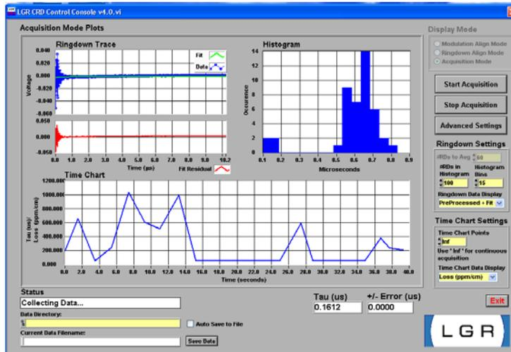
Fig.11 – Loss registration at 1 064 nm with  $\text{CO}_2$  for first 14 s ( $600 \text{ ppm/cm}$ ), two spikes of  $1\,000 \text{ ppm/cm}$ ,  $0.5 \text{ l/minute}$  flow rate. Flowing of  $\text{CO}_2$  is stopped after 14 seconds.
