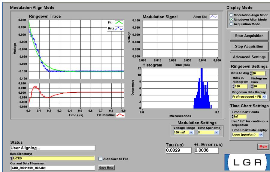
Fig. 7 – A screen capture with measurement for atmospheric air in cavity at 564 nm, 195 μs Q-Switch delay time,  $R = 99.8800@564 \text{ nm}$  (maximum is  $R = 99.9985\%@540 \text{ nm}$ ).
