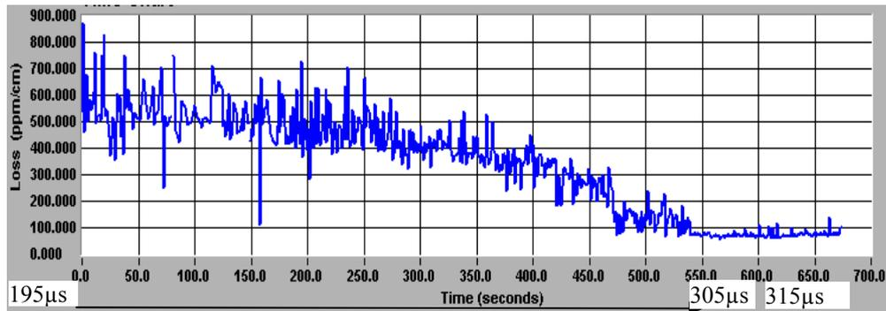
Fig. 6 – Total loss of cavity with CO<sub>2</sub> at 0.5 l/min continuous flow rate for a 660 s registration time, Q-Switch delay time ranging in 195–315 μs interval at 1 064 nm. Total loss are in  $70\text{--}600 \times 10^{-6} \text{ cm}^{-1}$  range for 25 °C, laser energy: 360 mJ (195 μs Q-S delay time) to 17 mJ (315 μs Q-S delay time) step of 10 μs at every 50 s measurement time.
