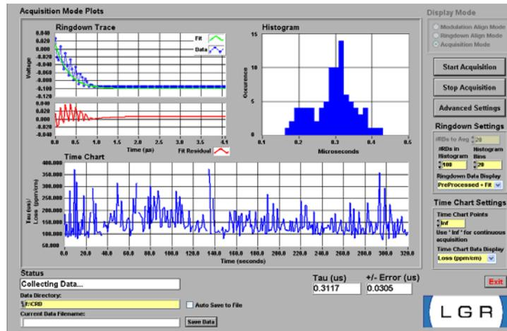
Fig. 8 – Measurement with atmospheric air in cavity at 564 nm, at a constant 260  $\mu\text{s}$  Q-Switch delay time,  $R = 99.8800@564$  nm, cavity loss = 105.87 ppm/cm.
