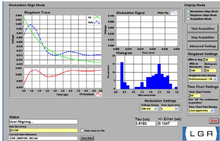
Fig. 9 – Measurement with atmospheric air in cavity at 564 nm, 307  $\mu\text{s}$  Q-Switch delay time,  $R = 99.8800@564$  nm.
