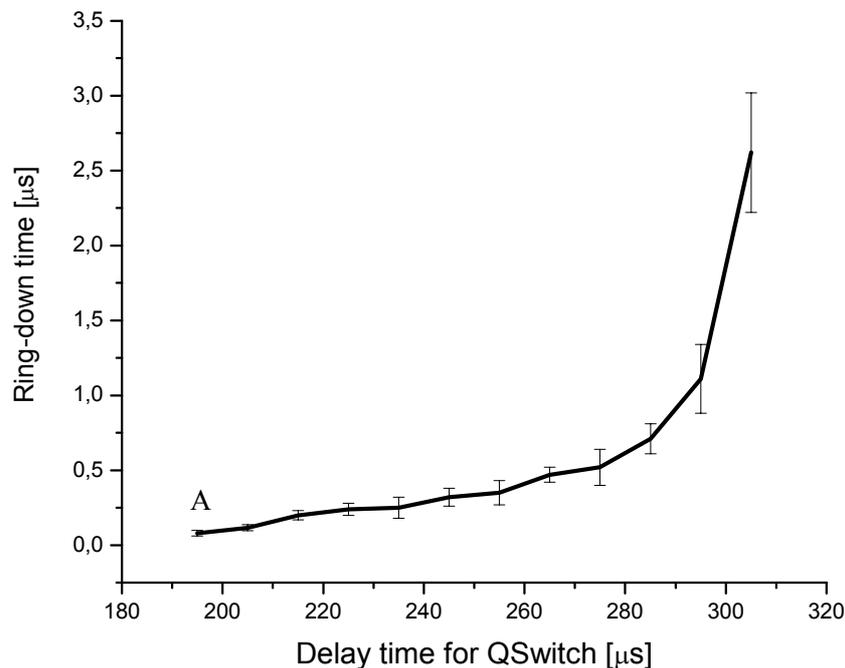
Fig. 3 – Ring-down time of laser pulse of 564 nm from RD cavity versus Q-Switch delay time of Brilliant laser.
