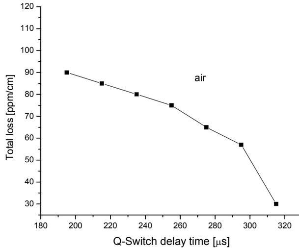
Fig. 4 – Total measured loss baseline versus Q-Switch delay time for air (1 atm.) in RD cavity at 564 nm pumping.
