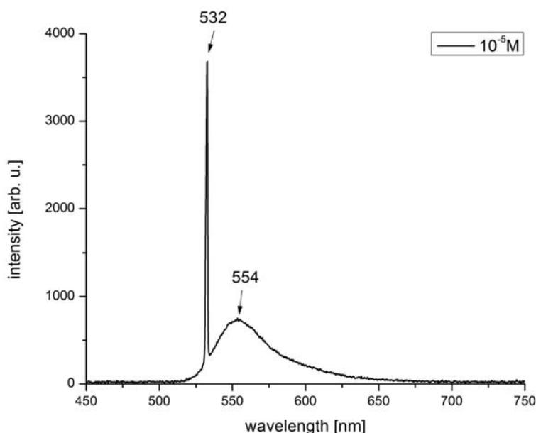
Fig. 11 – The fluorescence spectrum emitted by R6G ( $c = 10^{-5}\text{M}$ ) measured on a pendant droplet at  $10^{-5}\text{M}$  concentration.
