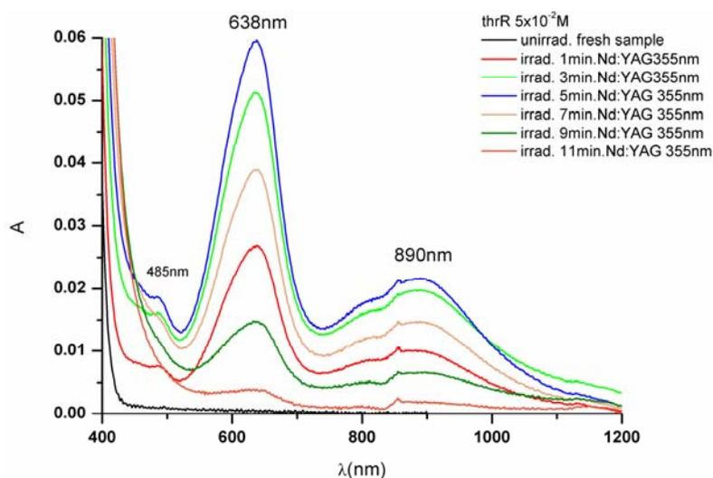
Fig. 8 – The absorption spectra of  $5 \times 10^{-2} \text{M}$  solution of Thr exposed to 355 nm Nd:YAG pulsed laser radiation.
