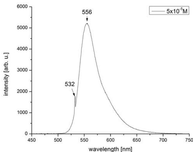
Fig. 12 – The fluorescence spectrum of R6G measured in droplet at  $5 \times 10^{-5} \text{ M}$ .
