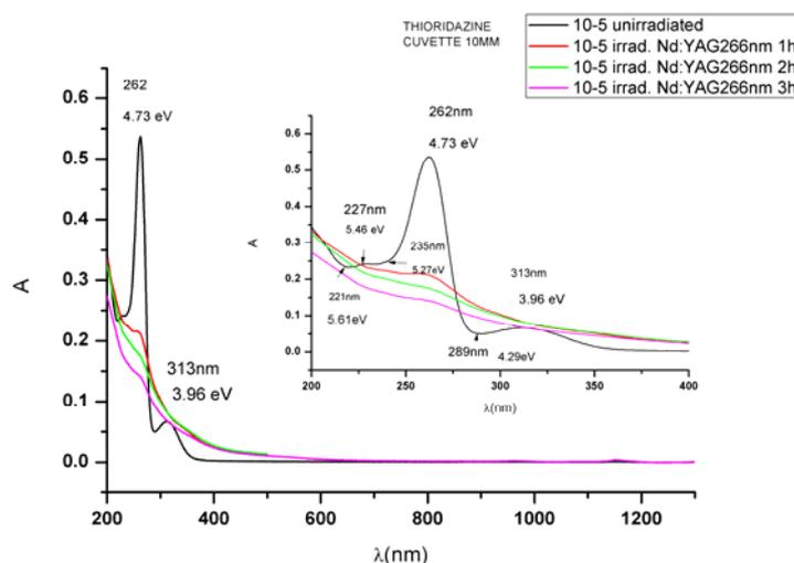
Fig. 6 – The absorption spectra of Thr  $10^{-5}$ M solution unirradiated and exposed to 266 nm Nd:YAG pulsed laser radiation.
