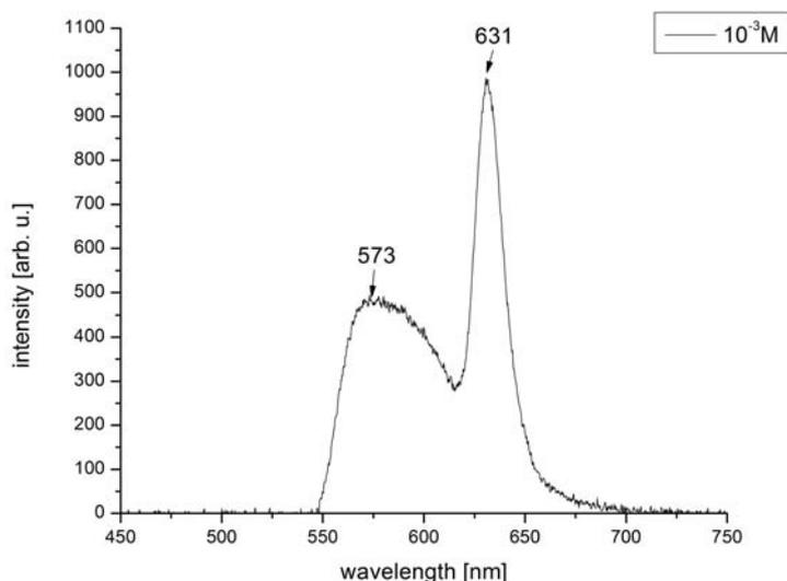
Fig. 14 – The fluorescence spectrum of R6G measured in droplet at  $10^{-3}\text{M}$ .
