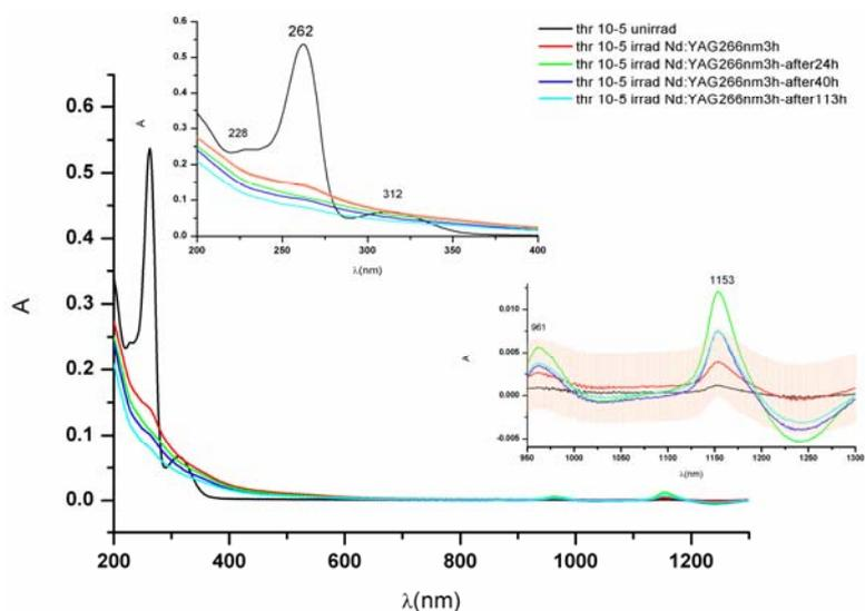
Fig. 7 – Time behaviour of the light absorption properties of Thr.
