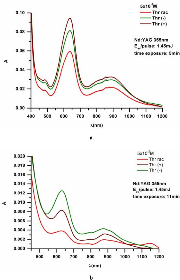
Fig. 10 – Comparison of absorption spectra of 5 min (a) and 11 min (b) irradiated Thioridazine solutions (rac / (-) / (+)).
