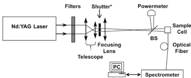
Fig. 2 – Laser irradiation experimental set-up: bulk exposure of compounds in sample cells (2.5 mL).
