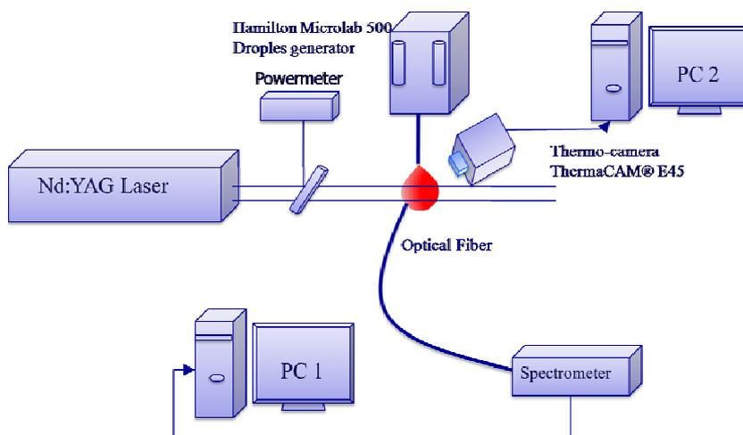
Fig. 3 – Experimental set-up.
