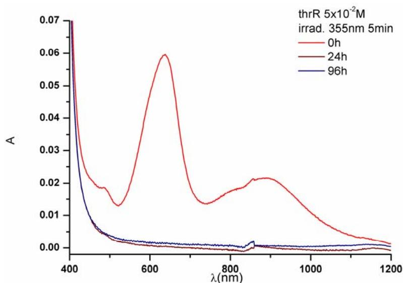
Fig. 9 – Time stability characterization of irradiated Thr solution.
