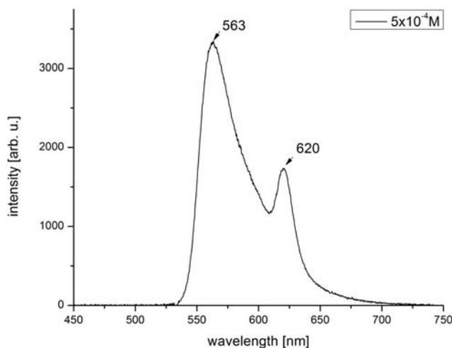
Fig. 13 – The fluorescence spectrum of R6G measured in droplet at the  $5 \times 10^{-4} \text{ M}$ .
