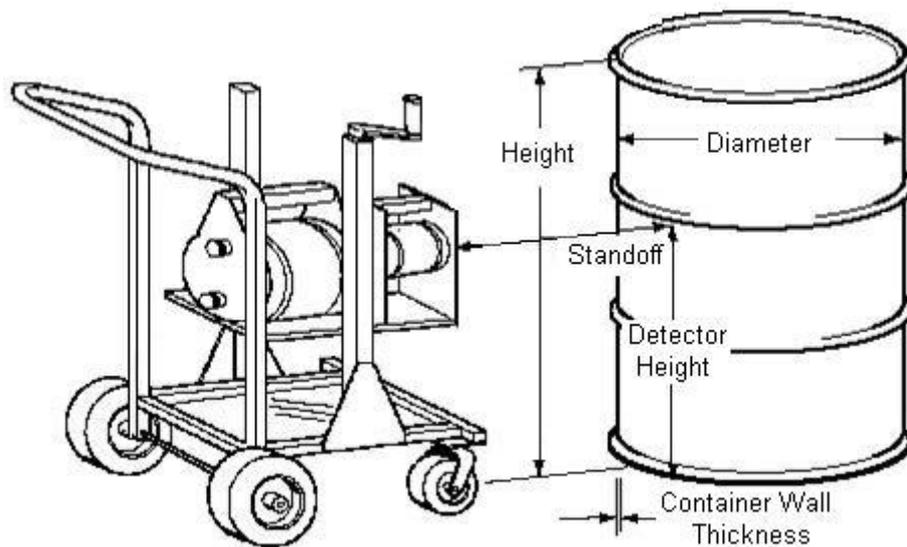
Fig. 1 – The ISOCART measurement geometry representation (from the ISOTOPIC Program for Radioactive Waste Characterization).
