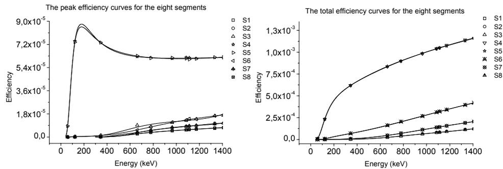
Fig. 3 – The peak (left) and total (right) efficiency curves for the eight segments.
