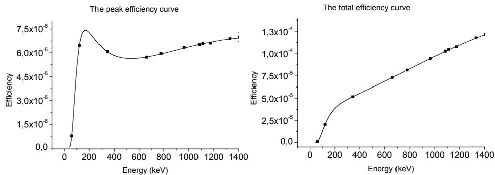
Fig. 4 – The peak (left) and total (right) efficiency curves for the drum .
