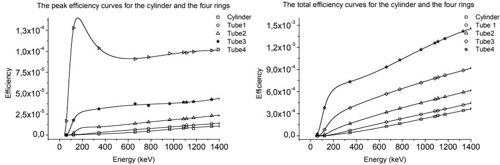
Fig. 2 – The peak (left) and total (right) efficiency curves for the cylinder and the four tubes.
