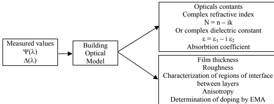
Fig. 2 – Characterization of physical properties by spectroscopic ellipsometry [1].
