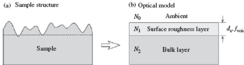
Fig. 4 – a) Sample with surface roughness; b) optical model composed of surface roughness and bulk layers. In (b),  $d_s$  and  $f_{void}$  represent the thickness of the surface roughness layer and the volume fraction of the ambient (voids) present within the surface roughness layer, respectively [1, 3].
