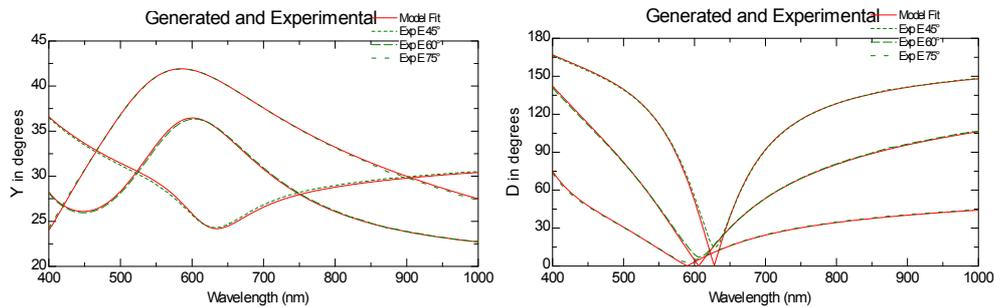
Fig. 3 –  $\Psi$  and  $\Delta$  configurations for 5Ni: YSZ and 10 Ni:YSZ thin films [4].
