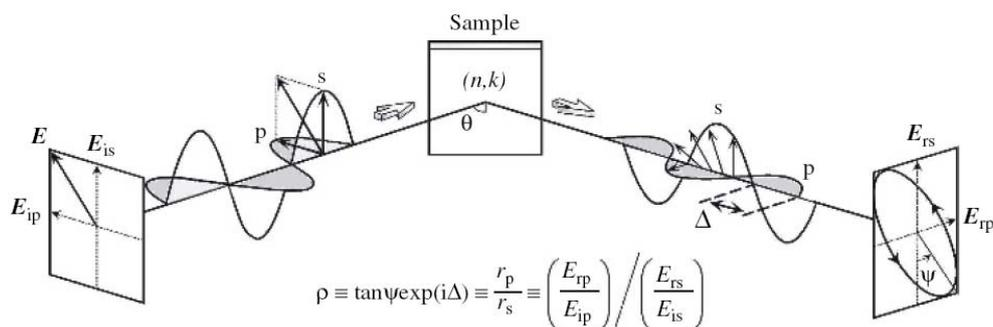
Fig. 1 – Measurement principle of ellipsometry [1].
