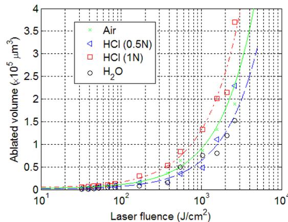
Fig. 3 – Dependence of the laser removed volume on the laser fluence in different ambient conditions.
