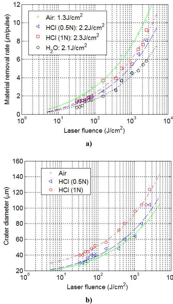
Fig. 2 – a) The removal rate vs laser fluence in different ambient conditions. The legend indicates the threshold fluences as resulted from extrapolation of the fitting curves towards zero removal rate;
