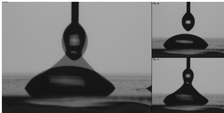
Fig. 2 – Ghost images: left – full interlaced frame; right – odd (up) and even (down) fields of the frame.
