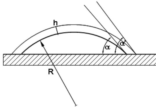
Fig. 5 – The effect of edge shift on estimated contact angle.
