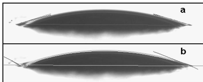
Fig. 8 – Influence of uncollimated lighting on estimated contact angles obtained with compared methods, for a test lens. The results of proposed algorithm are shown in the a): upper half of the picture; b) lower half shows the result of instrument's own software.
