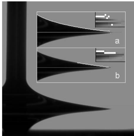
Fig. 9 – Behavior of edge detection algorithms near a cusp on drop profile. Inserts: a) – commercial software; b) – proposed method.
