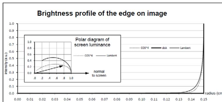
Fig. 4 – The dependence of brightness profile on lighting collimation, across the image of a reflecting sphere put in front of an illuminated screen.
