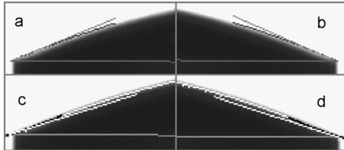
Fig. 7 – Influence of uncollimated lighting on estimated contact angles obtained with compared methods, for a test lens. The results of proposed algorithm are shown in the upper half of the picture. a, b – proposed method; c, d – commercial software.
