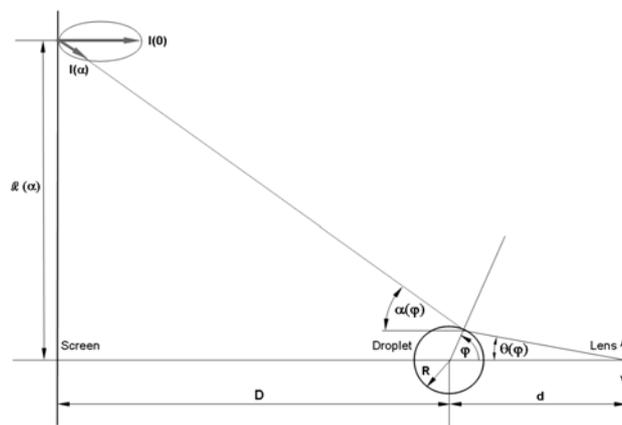
Fig. 3 – Geometry of light ray trajectories in a contact angle goniometer: The drop is represented as a sphere with radius  $R$ . On the left side there is the screen. The light comes from the left side and reflects on the drop surface towards the lens on the right side.
