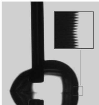
Fig. 1 – Jagged profile due to fast motion.
