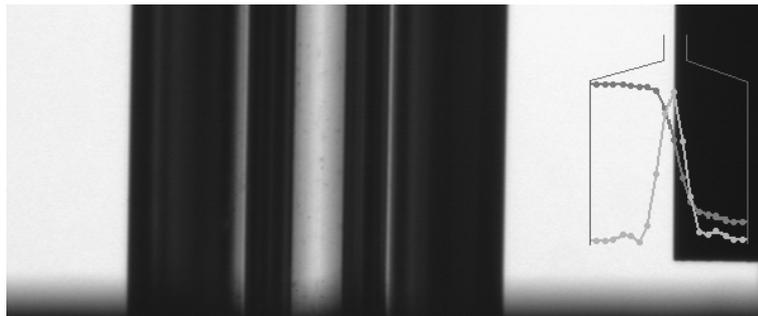
Fig. 6 – Glass rod (left) and razor blade (right) against a lit background. Overlaid are the brightness curve (dark gray) and its derivative (light gray), across the edge of razor blade.
