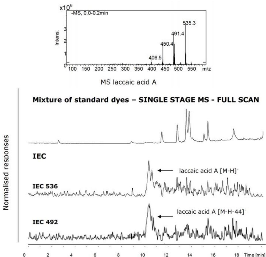
Fig. 3 – (top) MS spectra illustrating the molecular ion and fragments produced in the ionization source for a standard of laccaic acid A; (bottom) chromatograms obtained in Single Stage MS for a mixture of standards, also containing laccaic acid A; the IEC obtained for the molecular ion of laccaic acid A ( $m/z = 536$ ) and the ion produced by its decarboxylation in the ionization source ( $m/z = 492$ ).
