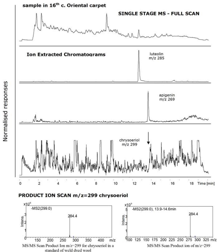
Fig. 1 – Flow chart diagram supporting the result obtained by MSD for a sample in a 16<sup>th</sup> c. Oriental carpet where *Reseda luteola* L. (weld) was identified.
