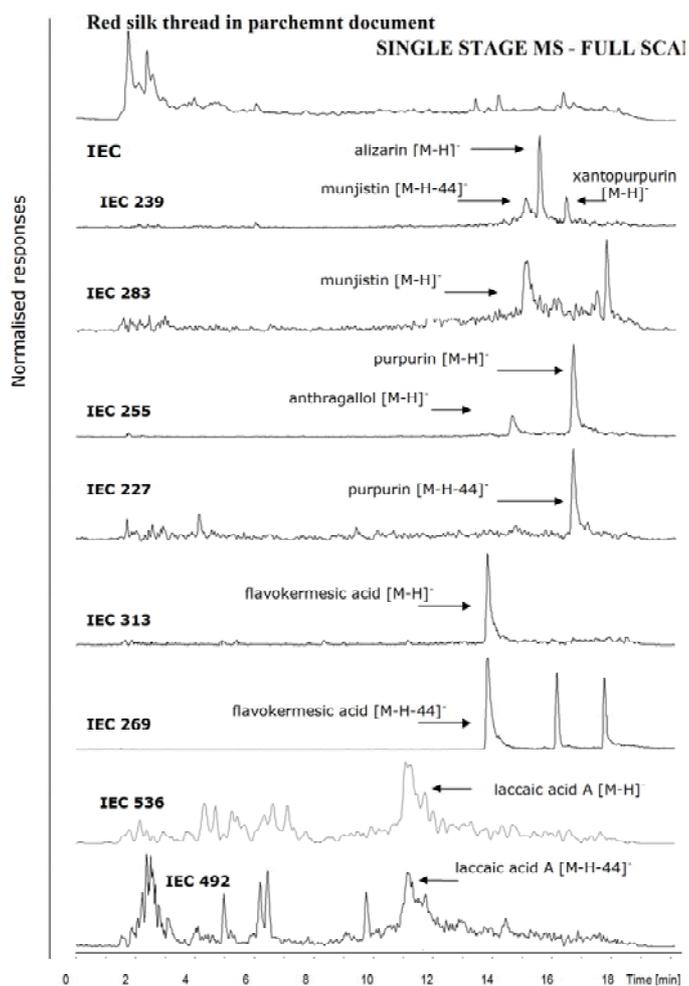
Fig. 2 – Flow chart diagram supporting the result obtained by MSD for a red silk thread sample from a parchment document where *Rubia tinctorum* L. (madder) and *Kerria lacca* Ker (lac dye) were identified.
