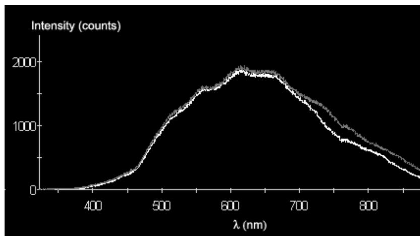
Fig. 7 – Emissions of an incandescent light bulb through air (gray) and through a layer of water (white).
