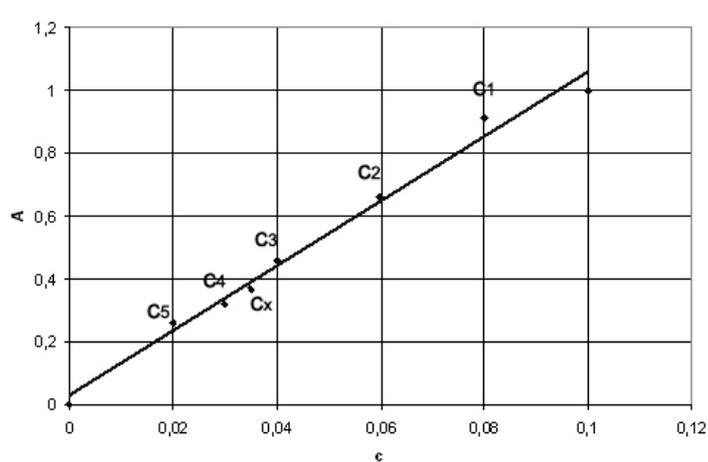
Fig. 11 – The absorbance dependence on concentration.
