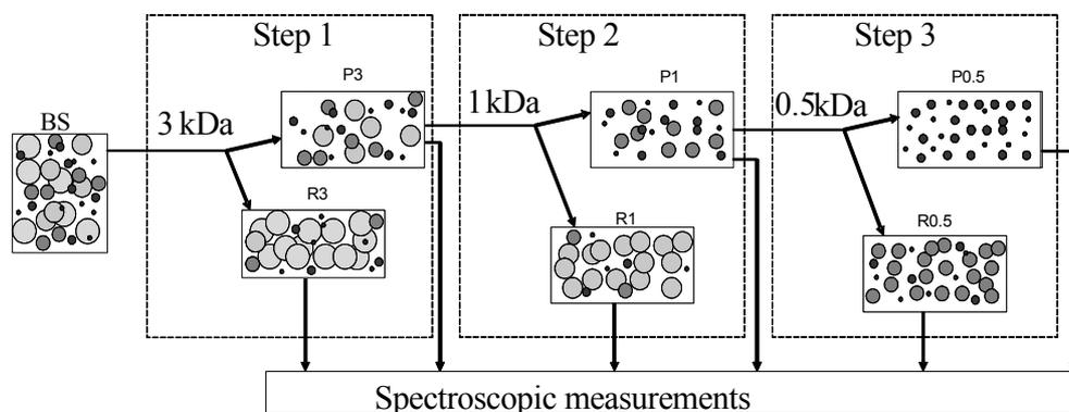
Fig. 1 – Working scheme for the ultrafiltration process.
