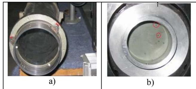
Fig. 7 – General view of the photosensitive plate, before (a) and after (b) the impact with the laser beam; several contact points impressed on the photosensitive plate are obtained.
