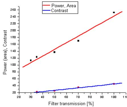
Fig. 14 – As the filter transmission is increasing, the power received is increasing too.
