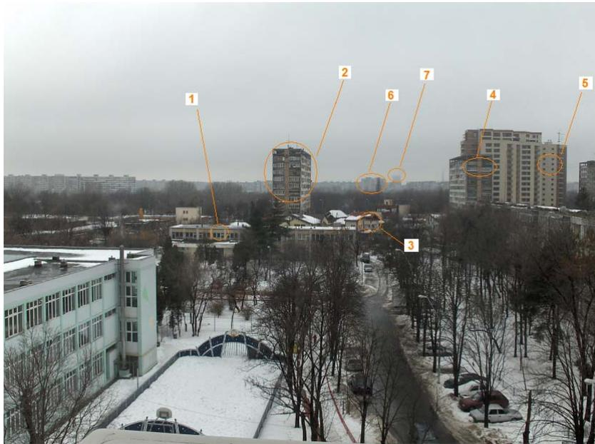
Fig. 8 – Example of an image acquired in normal atmospheric transparency for a winter day (visibility is 4,5 km); target 7 was the last possible rangefinder measured distance.
