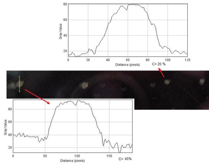
Fig. 13 – The image of the laser beam areas on the photosensitive plate when this surface is placed at a higher distance than the objective focal length; two contrast variation diagrams are given here as example.
