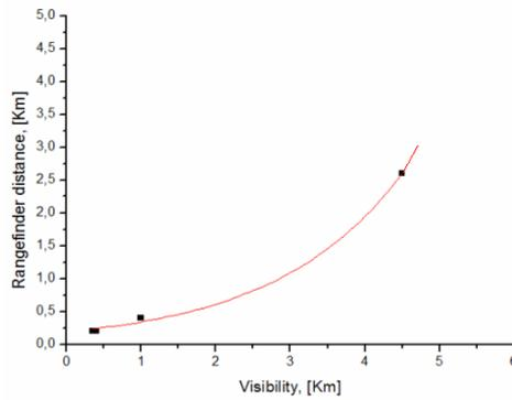
Fig. 16 – The rangefinder distance variation with visibility, in poor and medium atmospheric transmission.
