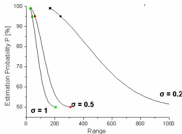
Fig. 5 – Range measurement probability estimated from the atmospheric transmission, expressed here by the attenuation coefficient  $\sigma$  [5].
