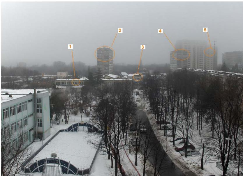
Fig. 9 – Example of an image scene acquired in lower atmospheric transparency (visibility is 1,4 km); target 5 was the last possible rangefinder measured distance.
