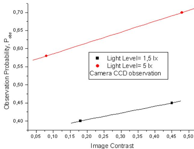
Fig. 20 – The observation probability is increasing with the image contrast of the target and with the light level.
