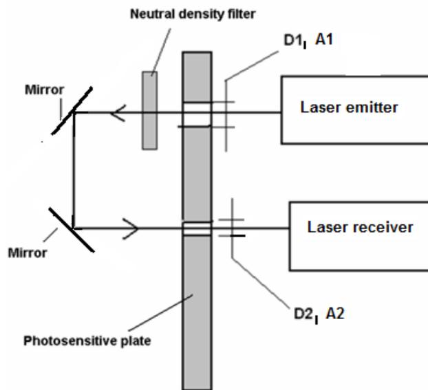
Fig. 6 – The scheme used to measure the powers ratio by measuring the areas  $A_1$  and  $A_2$  or diameters  $D_1$  and  $D_2$ .
