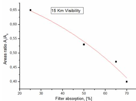
Fig. 15 – The areas ratio  $A_2 / A_1$  can estimate the rangefinder probability in normal visibility conditions.
