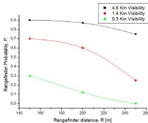
Fig. 17 – Rangefinder probability depends on the measured distance and the visibility conditions.
