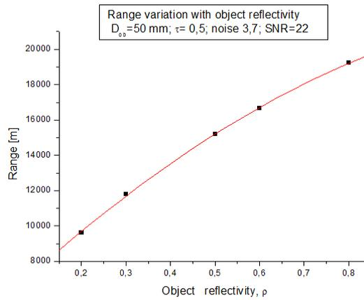
Fig. 4 – The rangefinder distance variation with object reflectivity;  $R_{\max} = R_{\max}(\text{rediffused power } \delta)$ .
