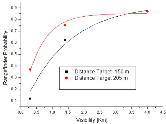
Fig. 19 – For different target distances, rangefinder probabilities may be different even for the same visibility.
