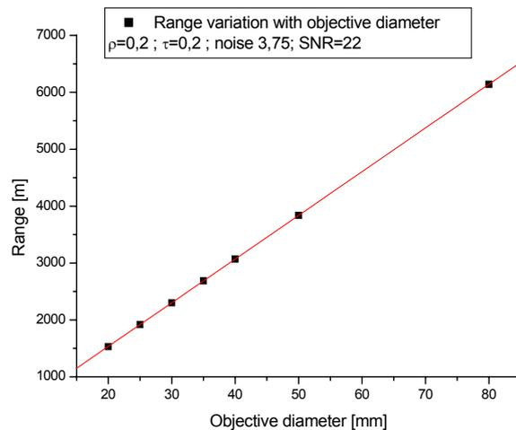
Fig. 1 – The rangefinder distance variation with objective diameter;
