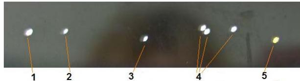
Fig. 12 - The image of the laser beam areas on the photosensitive plate when the surface is placed in the focal plane of the lens; the holes are as follows: 1 – without filter; 2 – with a filter of 30% transmission; 3 – with 35% transmission; 4 – with 52% transmission; 5 – with 75% transmission.
