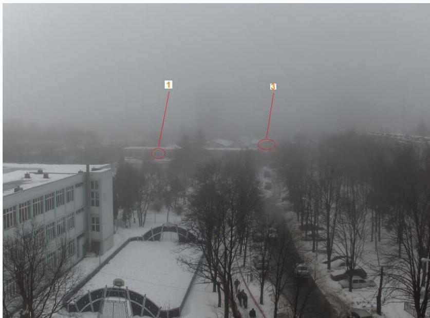
Fig. 11 – Example of the same image scene acquired in a much lower atmospheric transparency (visibility is 350 m); target 3 was the last possible rangefinder measured distance.
