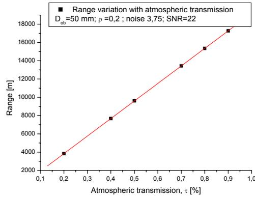
Fig. 2 – The rangefinder distance variation with atmospheric transmission;  $R_{\max} = R_{\max}(\tau_{\text{atm}})$ .
