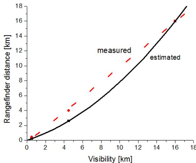
Fig. 18 – A correlation between the measured rangefinder distance and the estimated one in lab conditions can be made.
