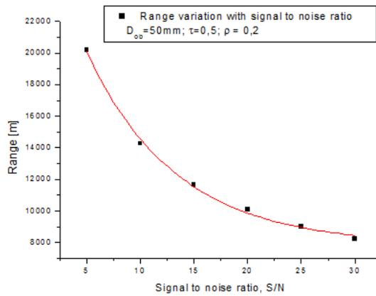
Fig. 3 – The rangefinder distance variation with signal to noise ratio;  $R_{\max} = R_{\max}(S/N)$ .
