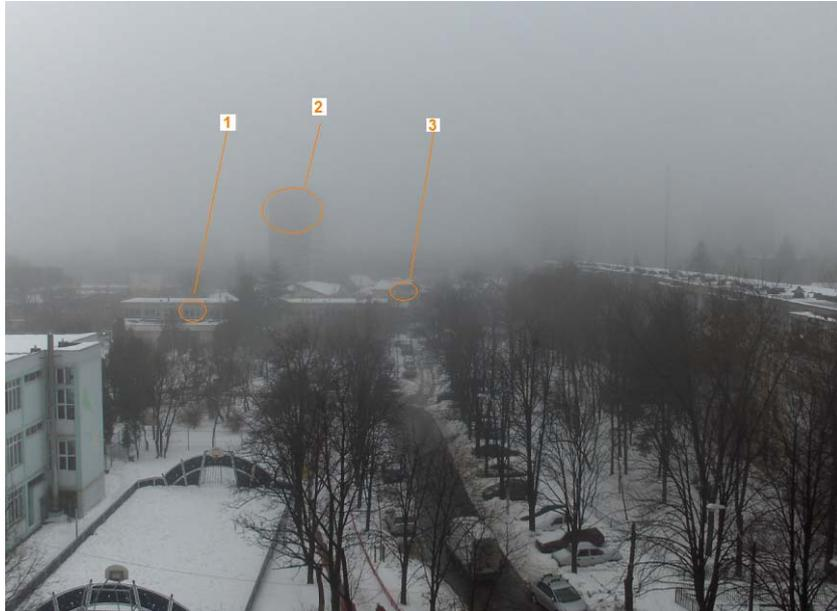
Fig. 10 – Image scene acquired in lower atmospheric transparency (visibility is 500 m); target 3 was the last possible rangefinder measured distance.
