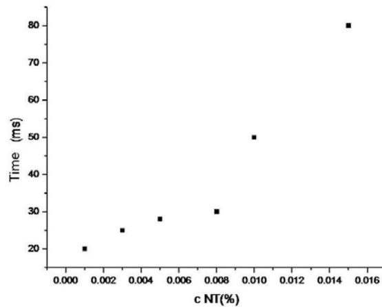
Fig. 5 – ON switching time dependence on the NT concentration ( $U = 15V$ ).
