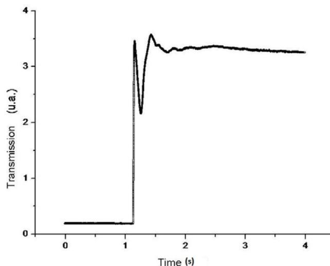
Fig. 3 – Electro-optical response of a liquid crystal E7 cell at applied voltage of 1.5V.
