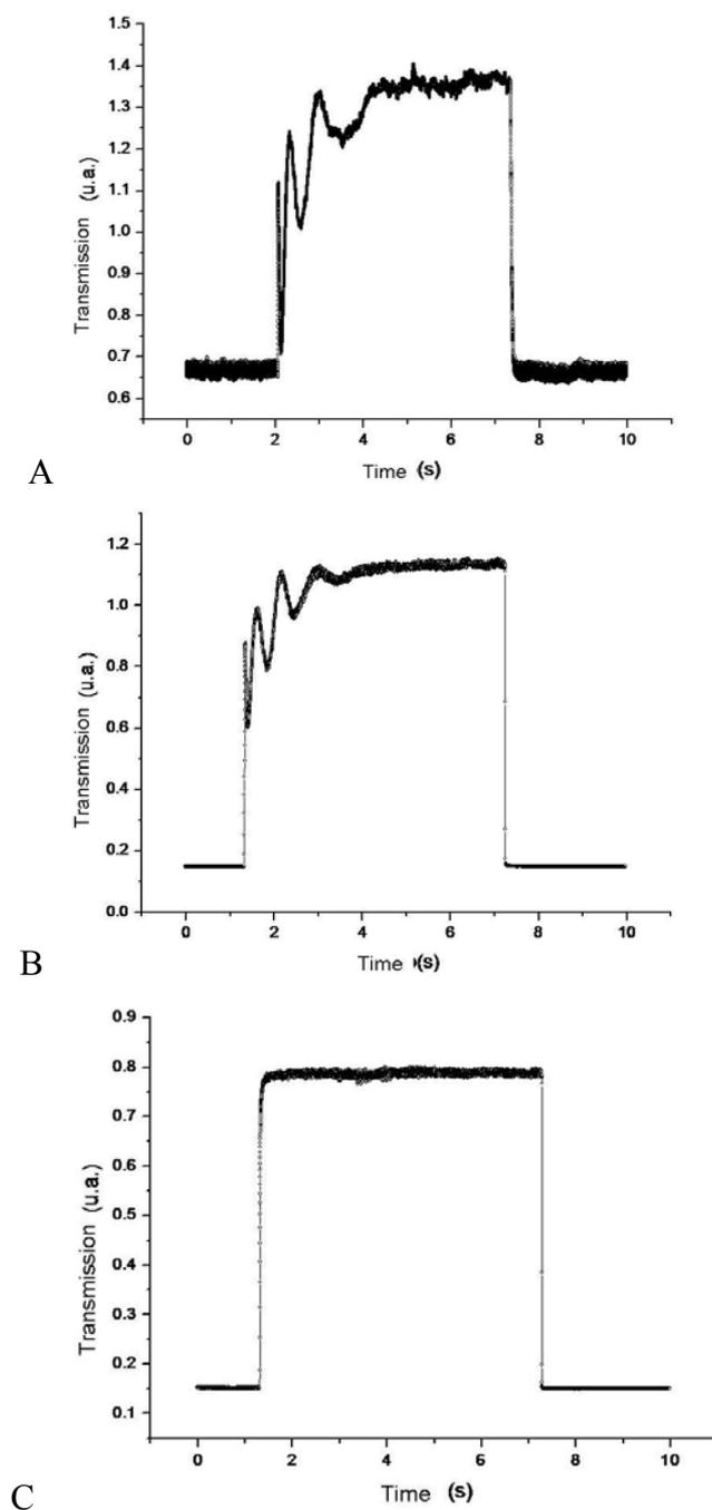
Fig. 4 – The form of electro-optical response of cells with E7 having different MWNT concentrations: A)  $c = 0.001\%$ ; B)  $c = 0.005\%$ ; C)  $c = 0.01\%$ .
