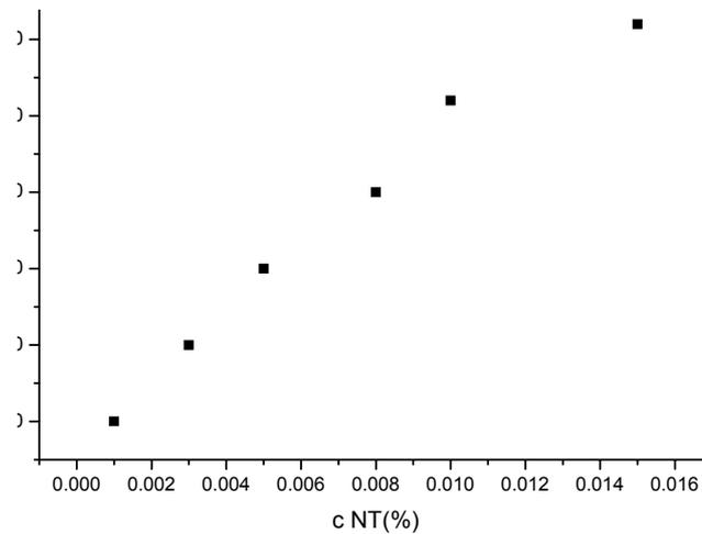
Fig. 8 – Delay Time induced by NT concentration ( $U = 15V$ ).
