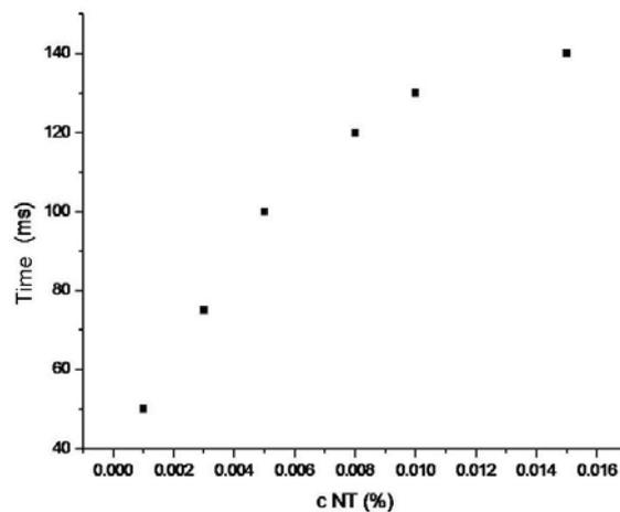
Fig. 6 – OFF switching time dependence on the NT concentration ( $U = 15V$ ).
