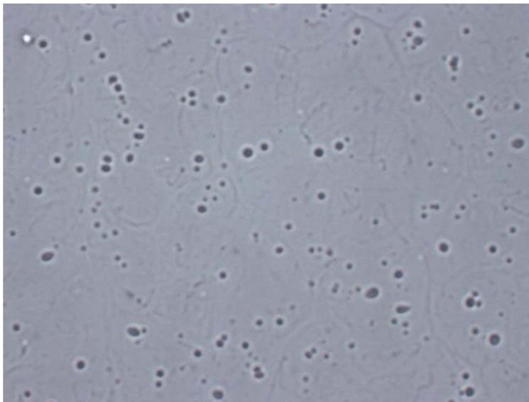
Fig. 2 – The view for the forming tendency of nanotubes SWNT clusters dispersed in liquid crystal E7,  $c = 0.01\%$ .
