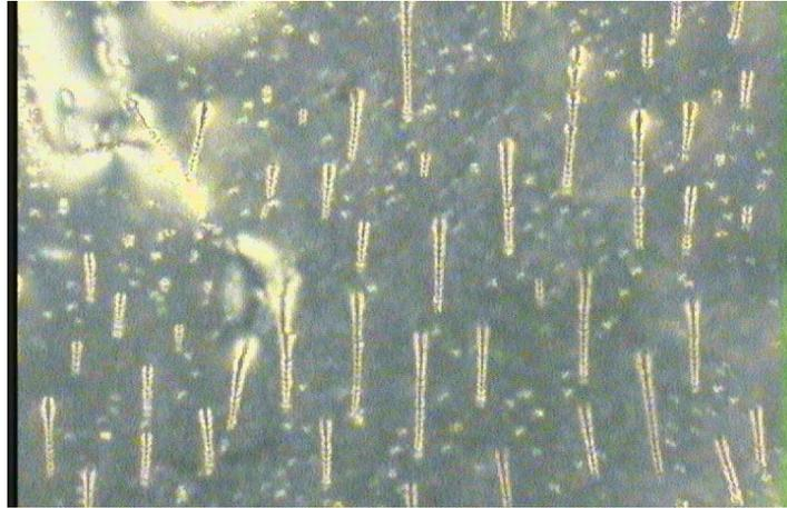
Fig. 1 – The view for the forming tendency of nanotubes MWNT fibrils dispersed in liquid crystal E7,  $c = 0.01\%$ .
